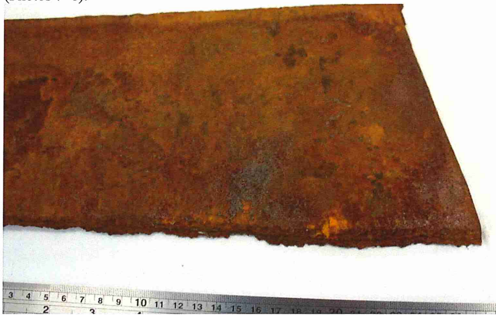
Photo 3. Torn edge of metal strip, view of hull exterior.
