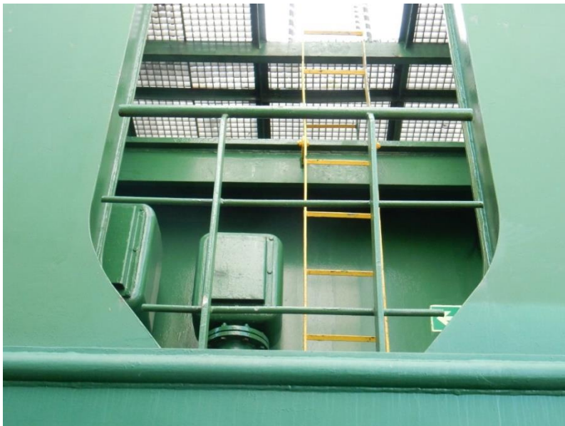
Figure 8. The ladder from deck to the grating, seen from the quay, i.e. from outside of the vessel.
