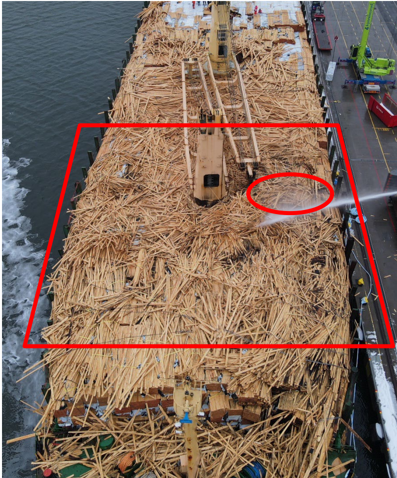
Figure 65. The square indicates the area in which the fire spread to varying degrees. The ring indicates the area that suffered the most extensive fire damage. The bow of the vessel is at the bottom of the picture.
