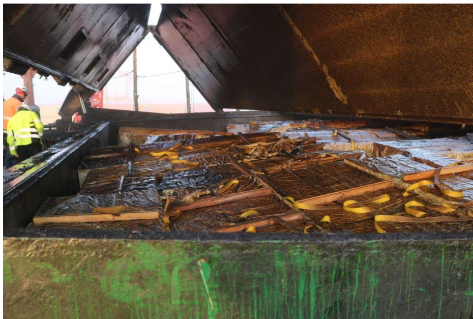
Figure 24. The timber cargo in cargo hold 1 when the hatches were opened and the deck cargo had been removed in Skandia Harbour in the Port of Gothenburg.
