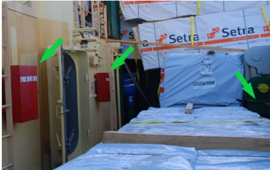
Figure 1. Example of the firefighting equipment on deck. The two arrows on the left mark the hose lockers and the right arrow marks the location of the fire hydrant. Timber was loaded between these.
