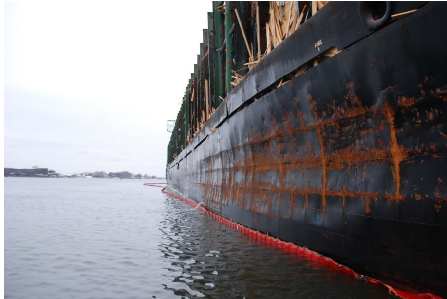
Figure 29. The hull damage on the starboard side.
