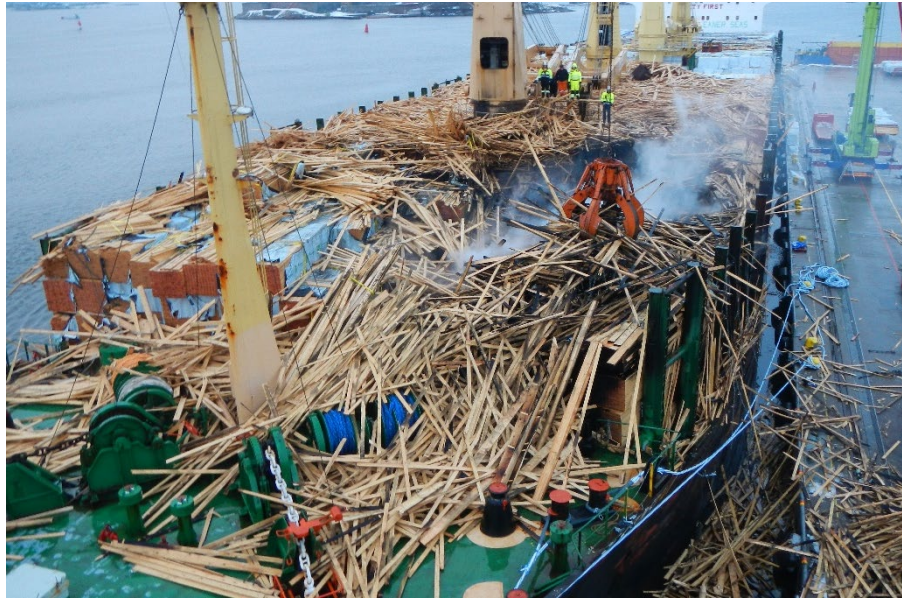
Figure 54. Unloading of the timber cargo in the fire area surrounding crane 1.
