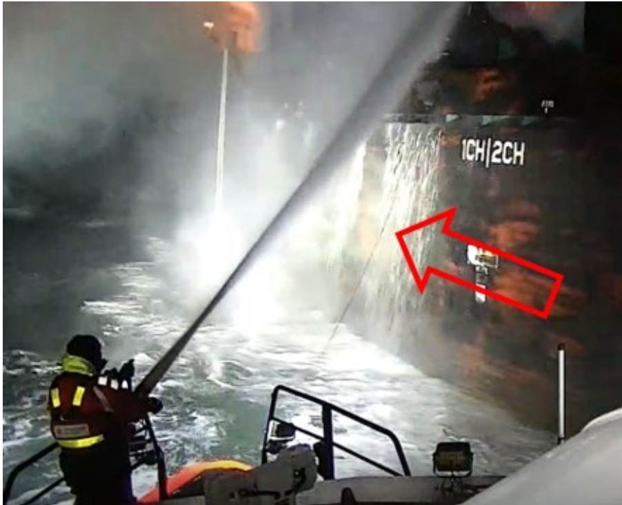
Figure 13. Image from the video recorded on one of the Swedish Sea Rescue Society's boats on Saturday 4 December. The arrow points to the extension cable that is probably the one that was torn off when the vessel departed from Orrskär.
