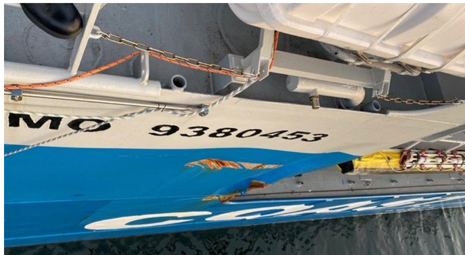
Figure 30. Damage to the port side of the vessel KBV 002. Image: Swedish Coast Guard.
