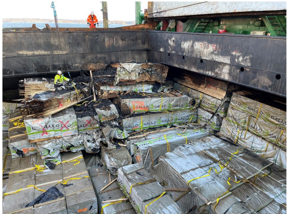
Figure 85. Cargo hold 1 during unloading in Lysekil. Some of the timber packages towards the port side of the cargo hold were heavily carbonised.
