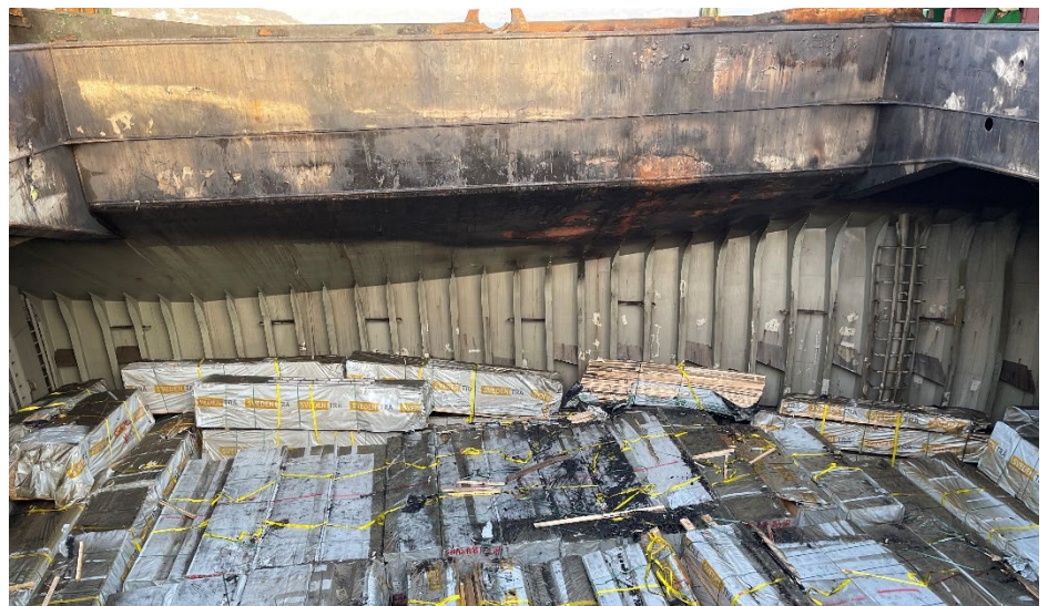
Figure 96. Soot and burned off paint on the port side of the cargo hold.
