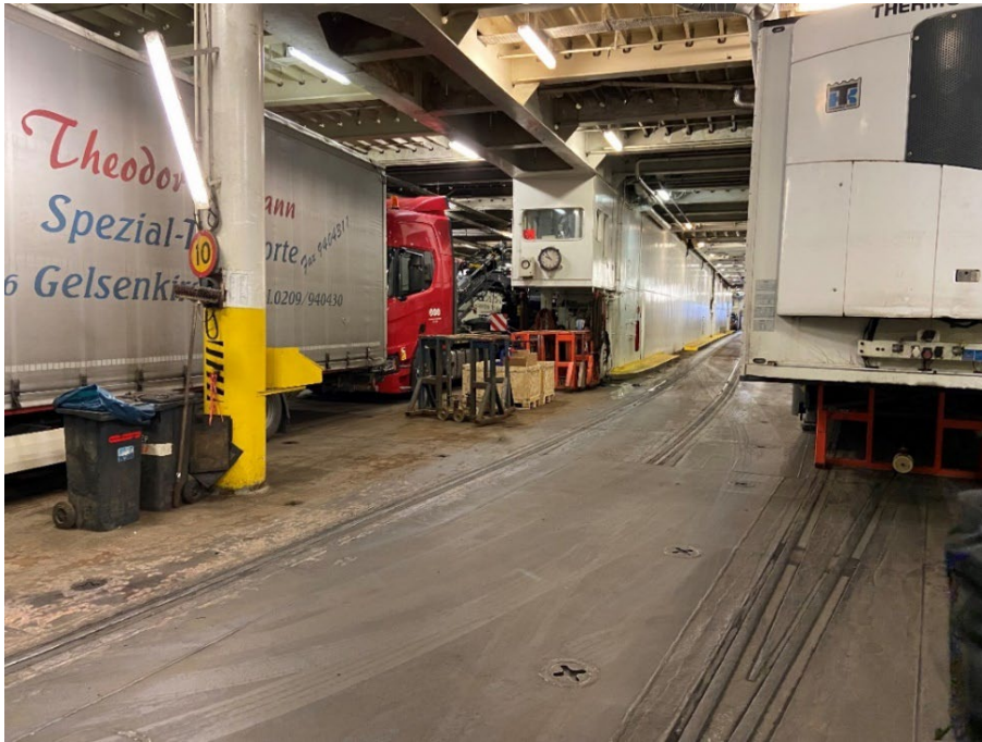
Figure 6. The picture is taken from the stern facing forward, in towards the car deck, and shows the pillar in the centreline and the aft edge of the centre casing where the electrical cables were hung.
