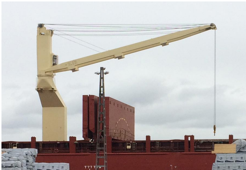
Figure 8. Ship crane no. 2 in the 32 m position. Lowest position for cargo handling. Cargo hatch covers in vertical position – means limited visibility into the second cargo hold. Image: MacGregor.
