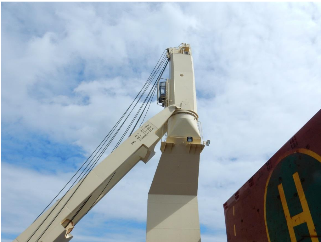
Figure 3. The ship's crane after the collapse.
