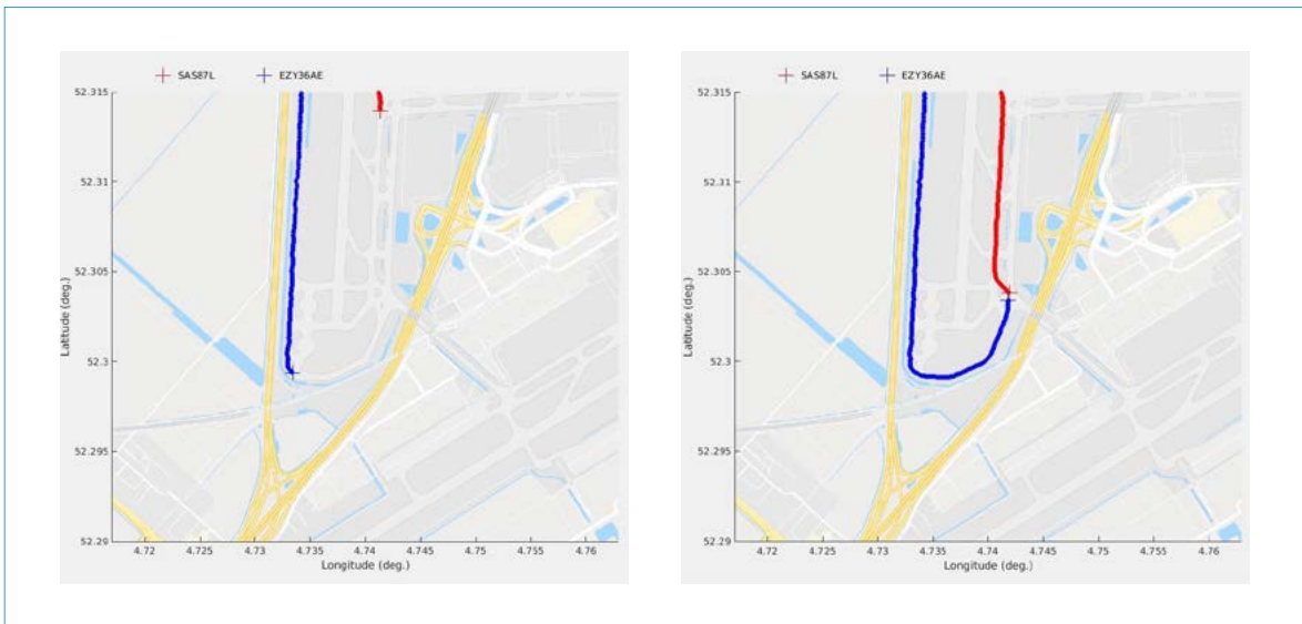
Figures 5a and 5b: positions of the aircraft at 19.36:01 and 19.37:30 hours respectively (Blue G-EZWY, red SE-DOY). (Source ATC the Netherlands)
