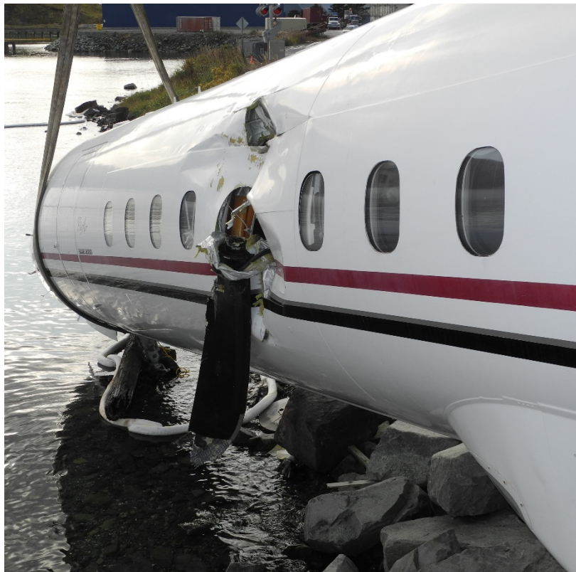
Figure 11. Impact area of left propeller blade.
