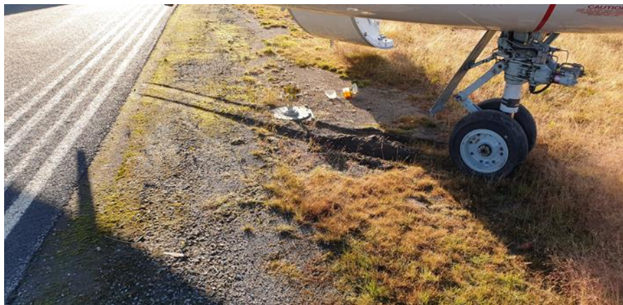
Figure 19. The aircraft came to a full stop with the nosewheel off the left side of the runway hard surface. Photo: The Rescue service Gällivare Airport.
