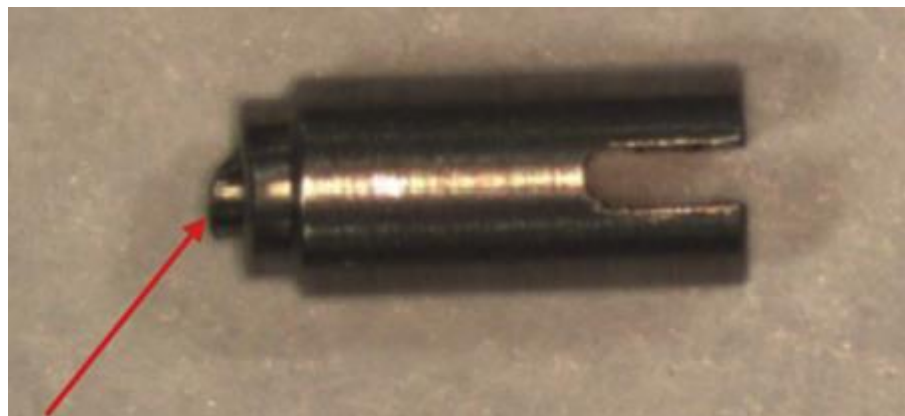
Figure 27. Hard stop that had been broken off and was loose in the stop cap assembly. The red arrow shows the fracture location.
