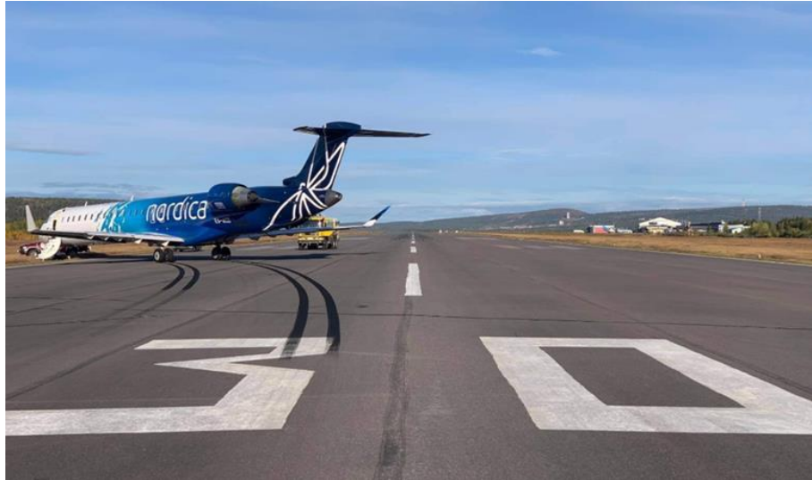
Figure 18. The aircraft's final position after the incident. After the runway marking 30, the black tire tracks are visible from the main wheels. Photo: The Rescue service Gällivare Airport.
