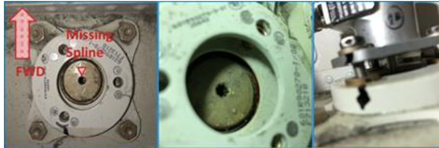
Figure 10. The photo to the left shows the pivot assembly with the sensor removed. The photo in the middle shows the depth to the splines from the flange on the pivot assembly. The right image shows the sensor partially installed. If the sensor is raised a little more from this position, the splined shaft will disengage from the pivot assy.
