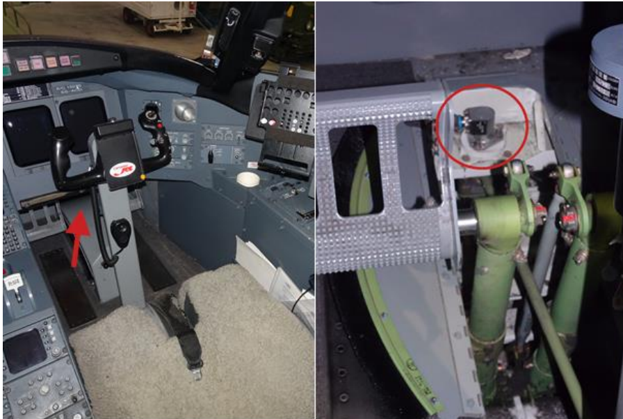
Figure 3. The picture on the left shows where the sensor is installed in the aircraft, in front of the rudder pedals on the right-hand side, see arrow. The picture on the right shows the sensor installed in the aircraft with panels removed.
