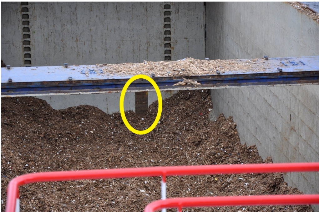
Fig. 3. The picture, which is aimed forward from the aft side of the cargo hold, shows the cargo hold after a large part of the cargo has been unloaded. The exit (marked yellow) from the forward shaft out into the cargo hold is seen in the middle of the picture. The wooden boards that are intended to prevent the cargo from getting into the shaft are still mounted in the tracks in the door hole. The inside of the door hole is seen in Fig. 4.
