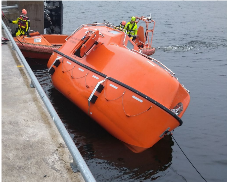
Figure 11. The list during the load test.
