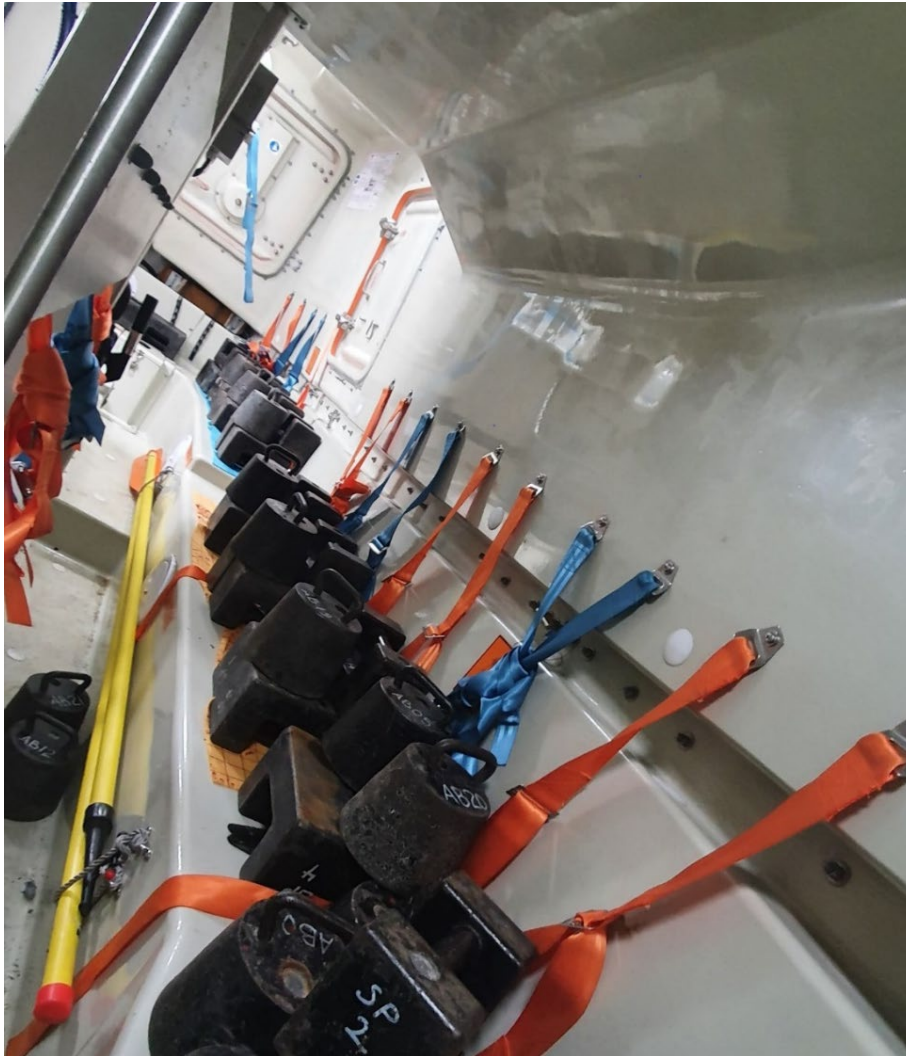
Figure 13. Picture from inside the lifeboat during the load test.
