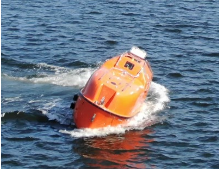
Figure 10. Picture from manoeuvring tests. Four people, including a helmsman, were on board. A sharp starboard turn was performed at a speed of 6 knots.
