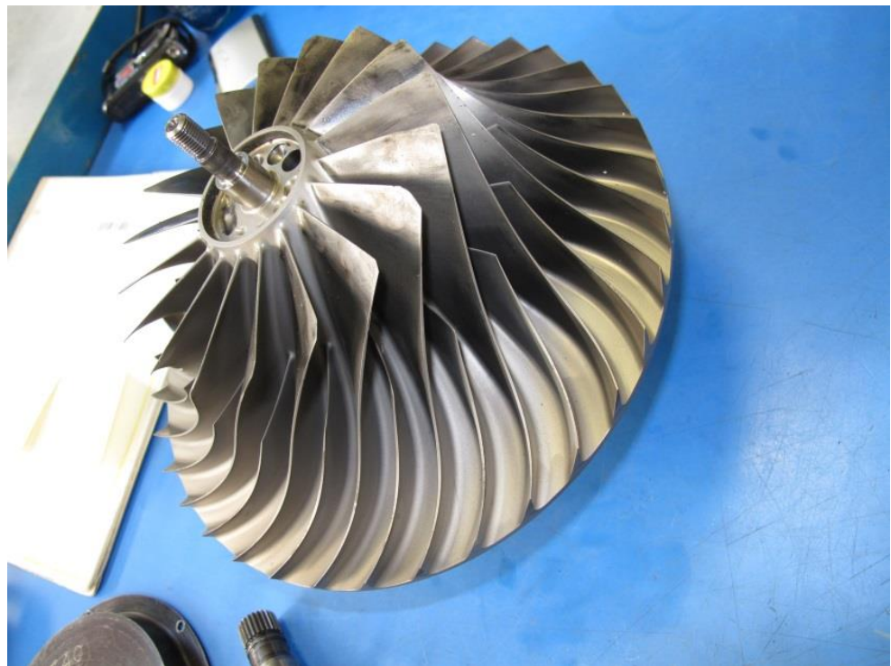
Figure 12. Radial compressor in good condition.
