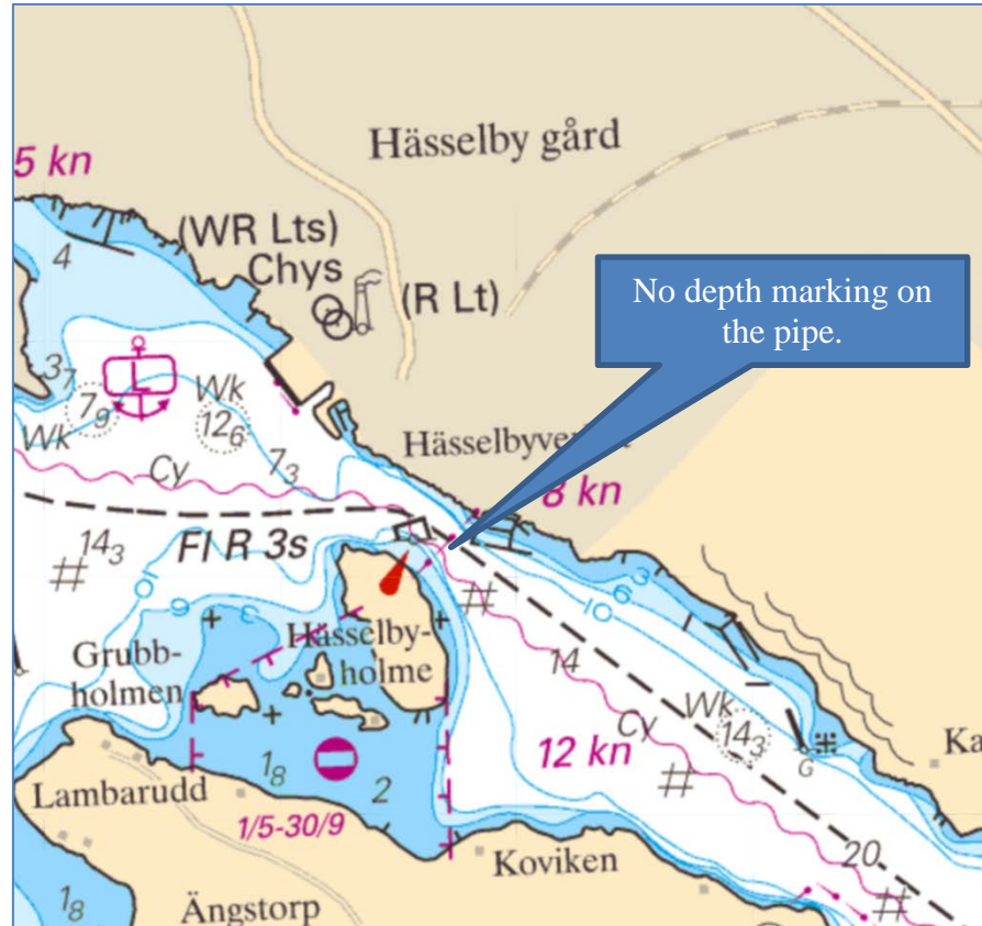
Figure 12. Hässelby holme and the marking of the water pipe. Image: The Swedish Maritime Administration's no. 10-01518 chart services.
