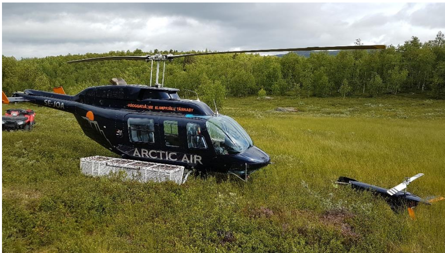
Figure 8. The site of the emergency landing, with the cut-off tail boom in front of the helicopter. Photo. The pilot.
