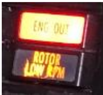
Figure 3. The indicators for engine failure and low rotor rpm are located furthest to the right on the caution/-warning panel.
