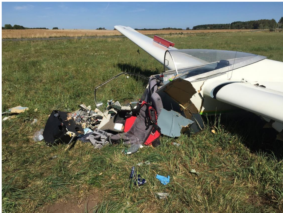
Figure 1. The front cockpit was severely demolished upon impact. Photo: Henrik Svensson.
