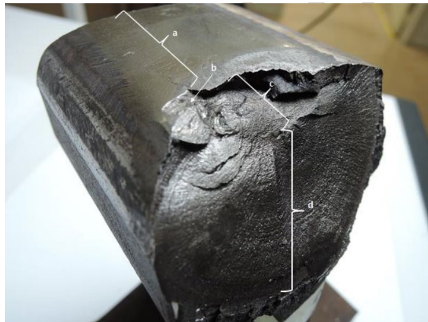
Figure 17. Fracture surface 1.2 showing the surface fatigue cracks (a), spalling (b), parallel crack (c) and vertical crack (d).
