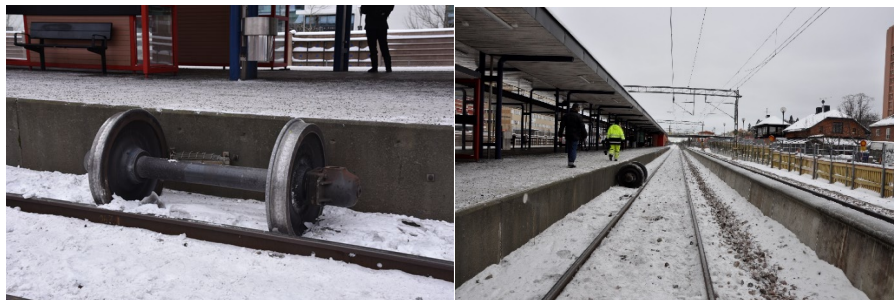
Figure 10. The final axle from the last freight wagon was found lying alongside the edge of the platform at Sollentuna commuter station, 600 metres after the broken rail.
