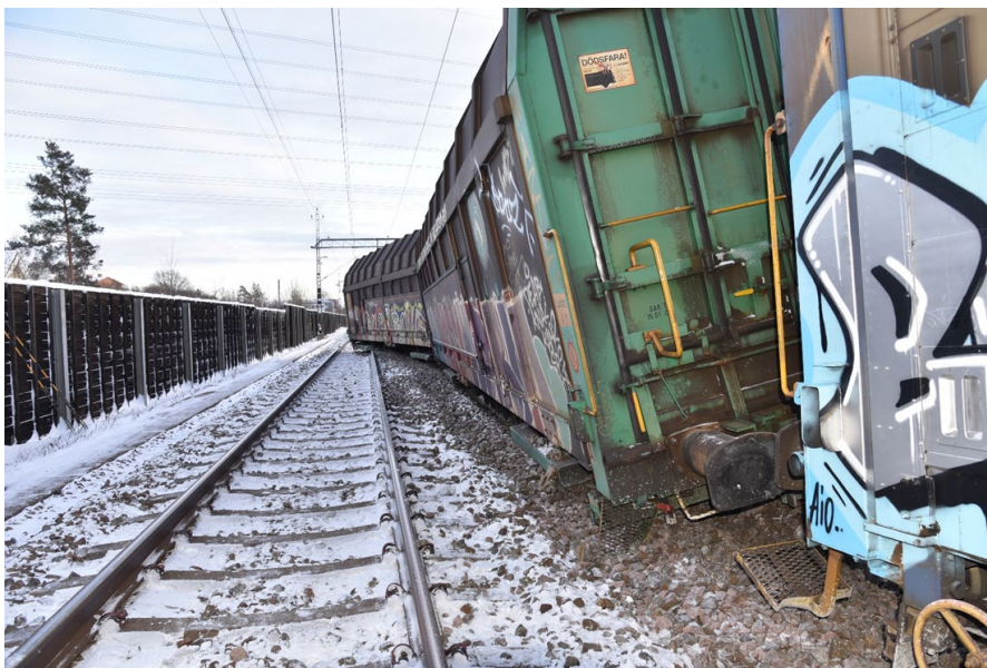
Figure 4. The last wagon came to a stop shifted sideways, with the rear portion in the adjacent track. The photographer is standing with their back facing in the train's direction of travel.
