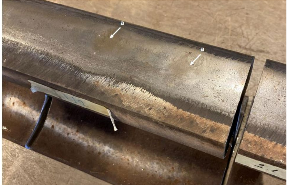
Figure 20. The running surface shows dark spots with surface cracking (a).
