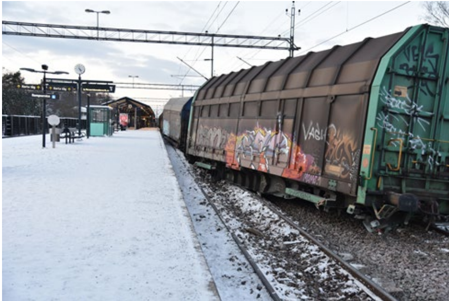
Figure 3. The train stationary following the derailment at Häggvik commuter station with the last wagon shifted sideways.
