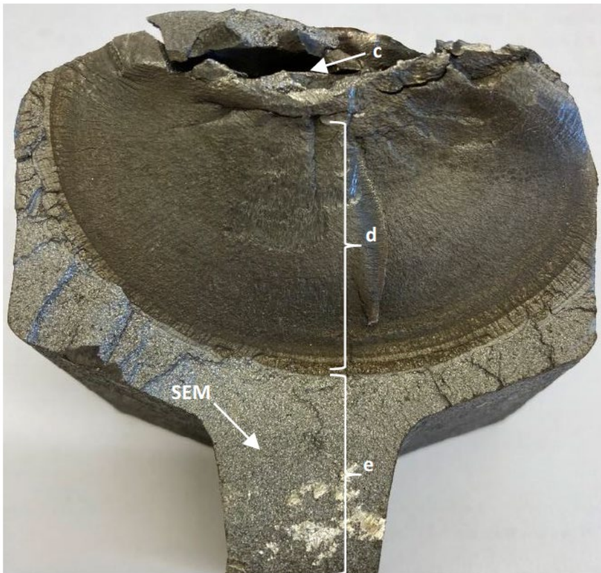
Figure 22. Fracture surface 1.1 with parallel crack (c), vertical crack (d) and overload zone (e) and the area investigated with scanning electron microscope (SEM).
