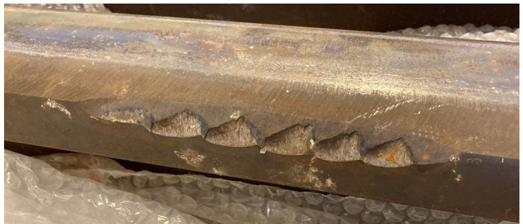
Figure 21. Mechanical damage between fracture surface 8.2 and 9.1.
