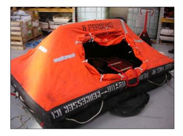
Picture of the raft - taken during a test of the inflation system at Raffel & Co in Denmark.
