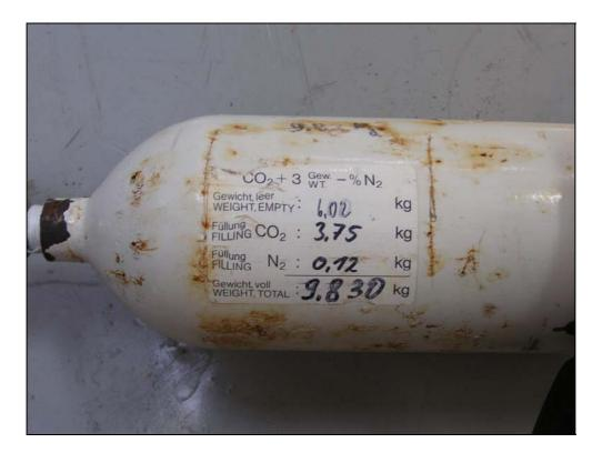
The raft's CO<sub>2</sub> bottle was according to its markings manufactured in 1990 and was pressure tested in October 2002. According to the marking and the re-inspection certificate, the gas mix was 3750, gr. of CO<sub>2</sub> and 120 gr. of N<sub>2</sub>.
