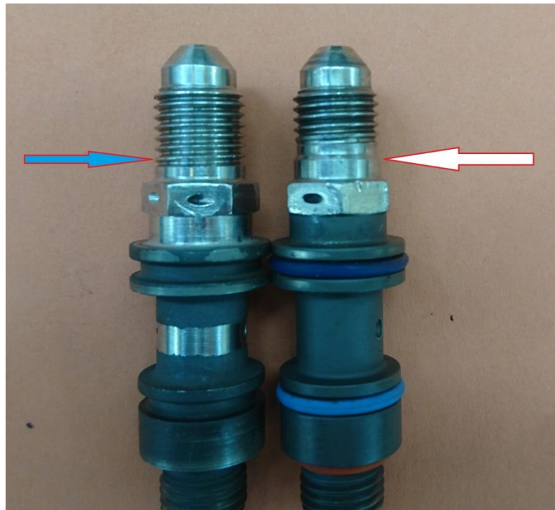
Figure 19. The inspected connection unit to the right and a reference connection unit to the left.
