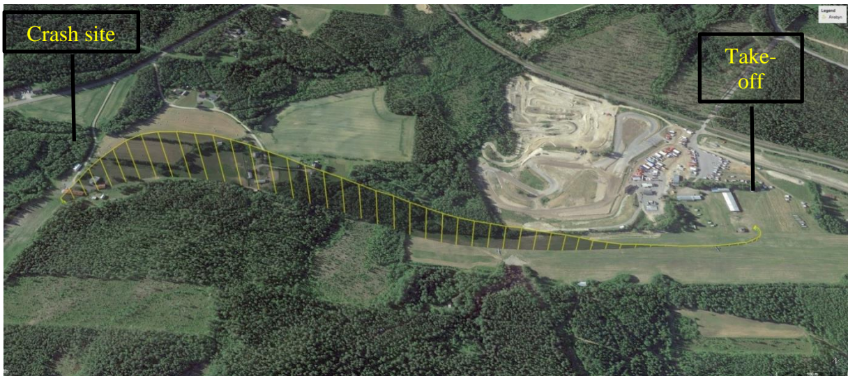
Figure 1. Flight path according to GPS data in the SkyDemo, presented in Google Earth. Älvsbyn/Högheden Airport can be seen on the right side of the image. The yellow columns show the approximate height above the terrain.
