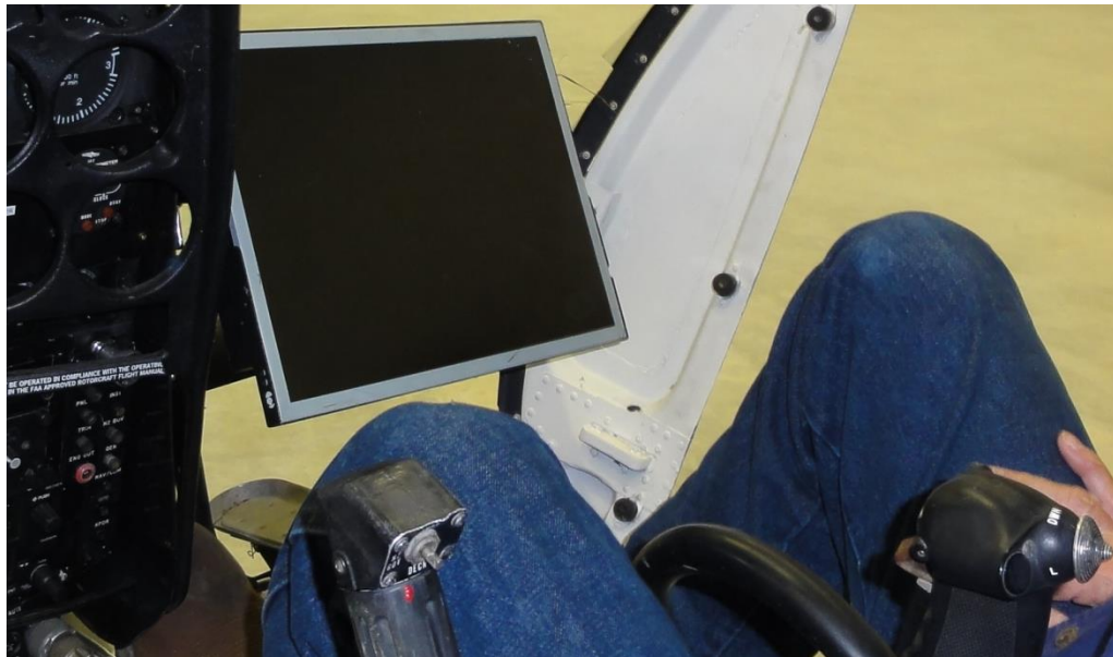
Figure 13. The field of view to the right and downwards as seen from the pilot's position, with the screen of the measuring system in place.
