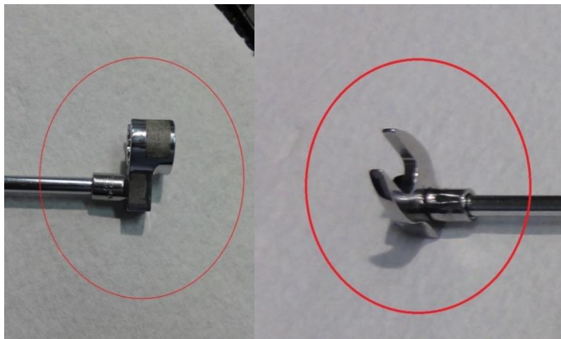
Figures 10 and 11. The flare-end and open-end (Also known as Crow foot) adapters used to install the pipe nut.
