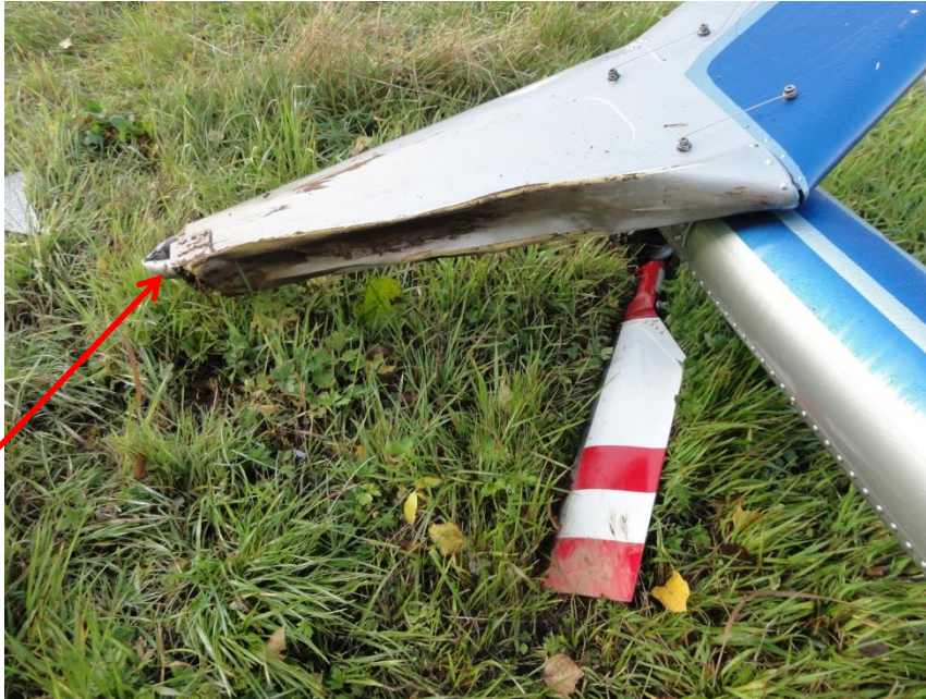
Figure 17. Ground contact with tail rotor guard and fin.
