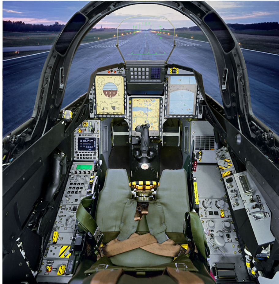
Figure 16. Gripen C cockpit. Navigation display in the centre with HUD above and in front of the front windscreen. Photo: Saab AB.
