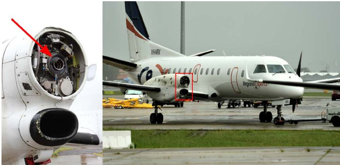
Figure 1: The aircraft, VH-NRX, at Sydney Airport after the incident showing the point of separation of the propeller in close-up
