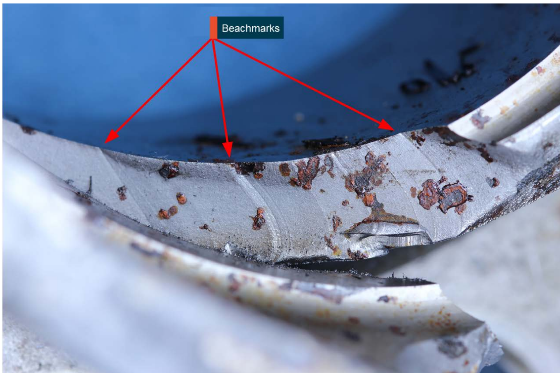
Figure 5: Section of the exposed propeller shaft showing beachmarks
