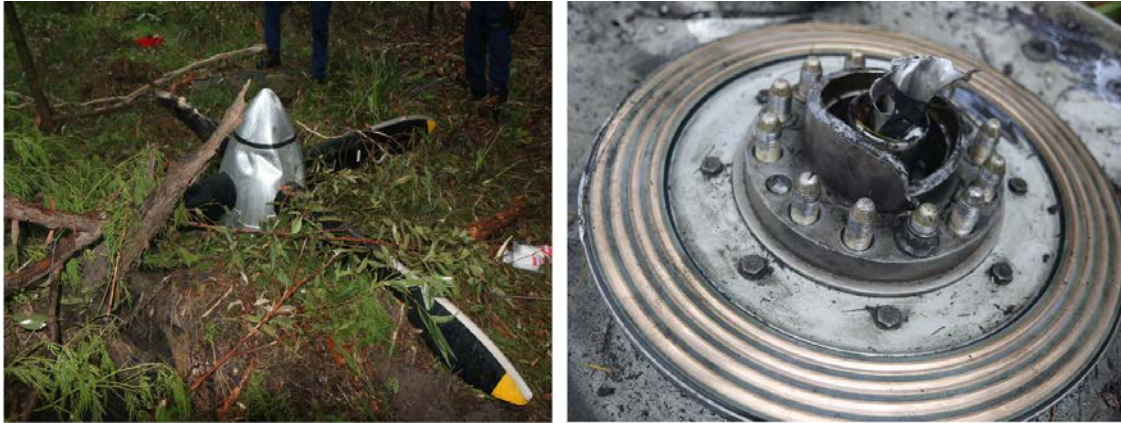
Figure 2: The separated propeller from VH-NRX
