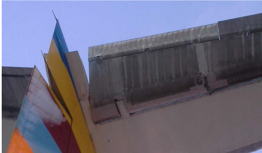
Figure 3. The rudder and right elevator after the incident. (Photo Aviator).
