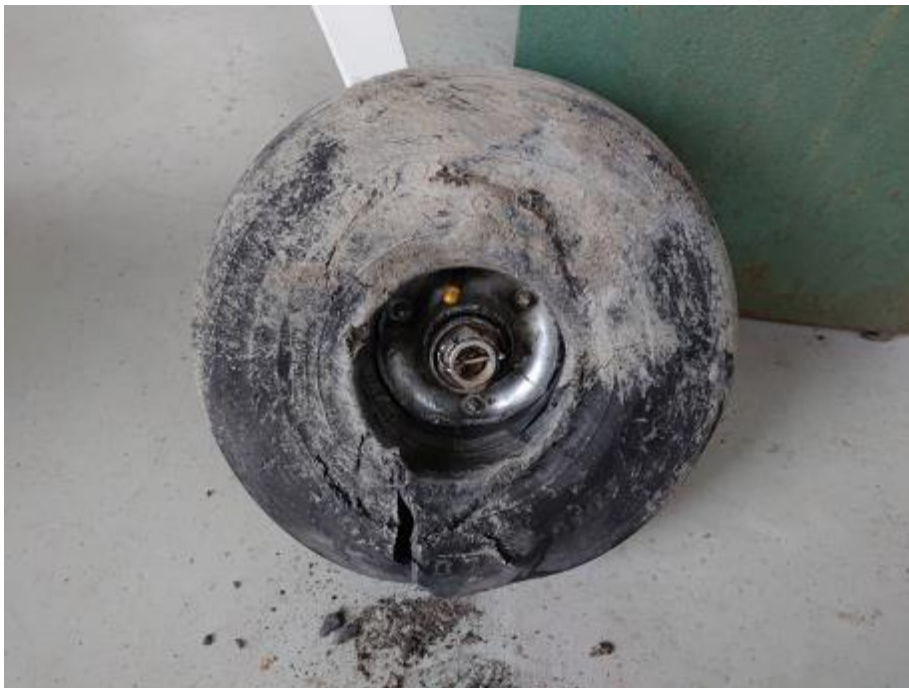
Figure 23. Damaged right wheel.
