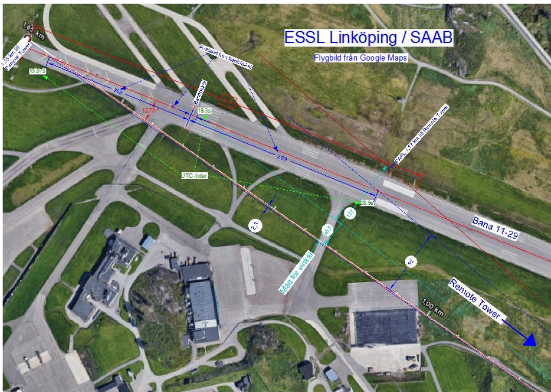
Figure 29. Lines drawn on image to calculate the aeroplane’s ground speed. Source: Google Maps with SHK added graphics.
