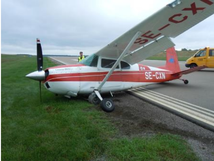
Figure 18. Right landing gear folded under the fuselage. Photo: Saab fire and rescue service.
