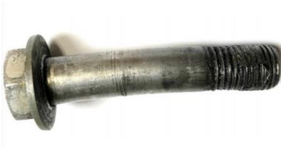
Figure 25. The bolt for attachment of the landing gear.
