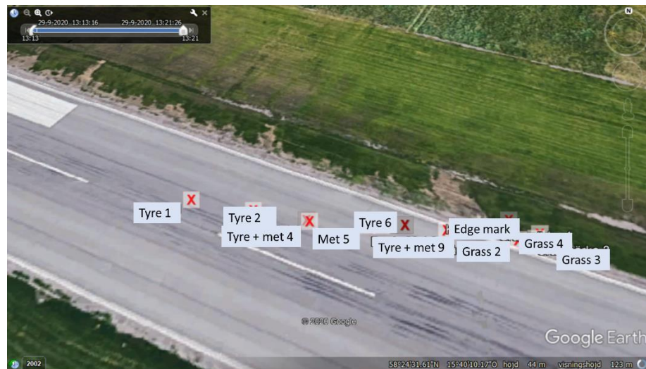
Figure 17. Marks on the runway from the first mark to the final position north of the runway (tyre and metal). SHK's measurements overlaid on a picture of the runway from Google Earth.
