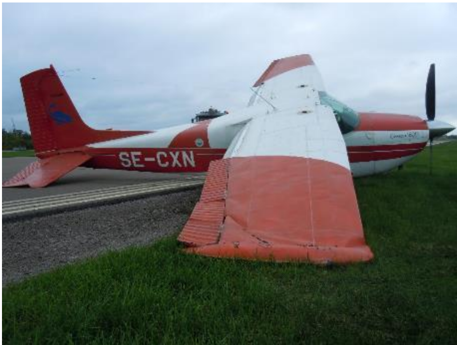
Figure 19. Damage to the right wing and aileron. Photo: Saab fire and rescue service.
