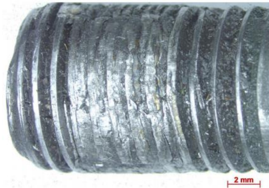
Figure 26. Enlargement of the bolt with deformed threads and metallic material in the threads.
