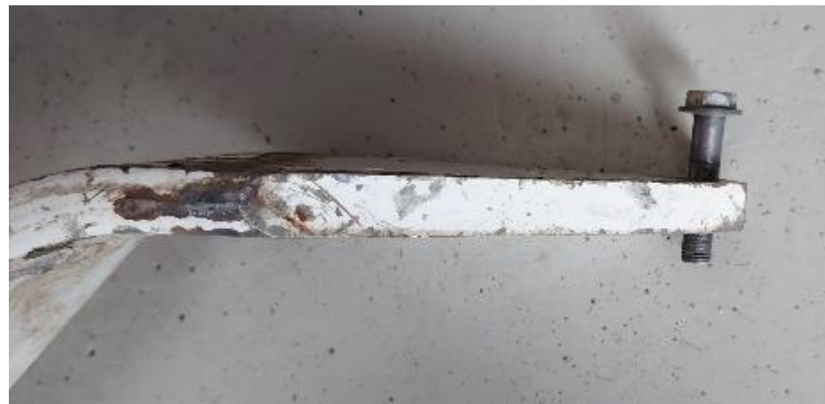
Figure 21. Landing gear strut with bolt for attachment.
