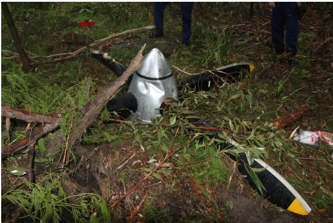
Figure 2: The propeller that had separated from VH-NRX as found by PoIAir about 8NM south-west of Sydney airport.
