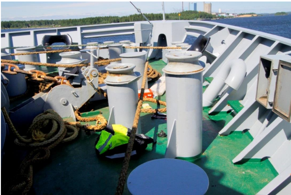
Fig. 6, Forecastle deck. To the right: the position of the chief officer when the accident occurred in the area of the platform at the remote control unit. To the left; the remaining of the parted spring line, piled up at its winch drum. It should be noted that the displayed configuration of the lines was made to moor the vessel after the accident and thus no representation of the common configuration used.
