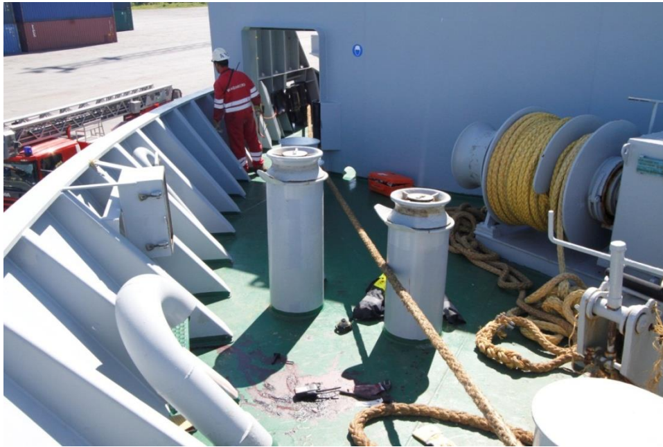
Fig.7, Forecandle deck, opposite direction. Through the opening in the bulkhead the spring line roller fairlead can be seen. It is likely that the spring line was lead over both of the pedestal fairleads seen in the middle of the picture. According to the pilot this was, despite the difference in height of the fairleads, the common way to run the spring line in the vessel series that Morraborg belonged to.
