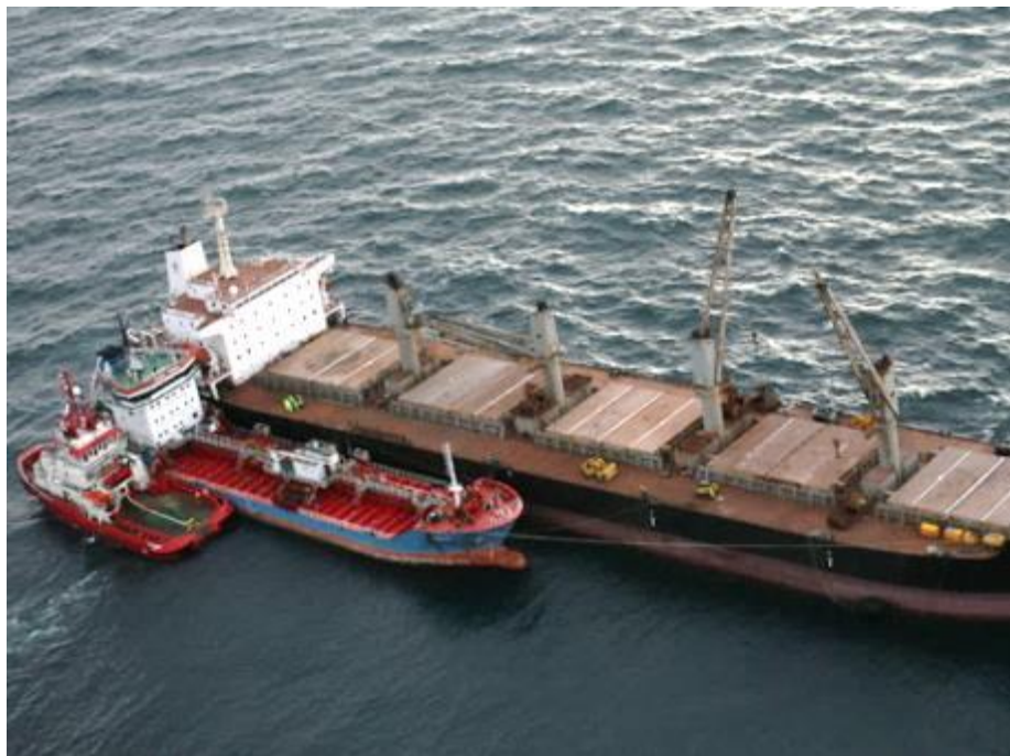
Figure 14. VICTORIA lightering bunker fuel to LEON. Image: The Swedish Coast Guard.
