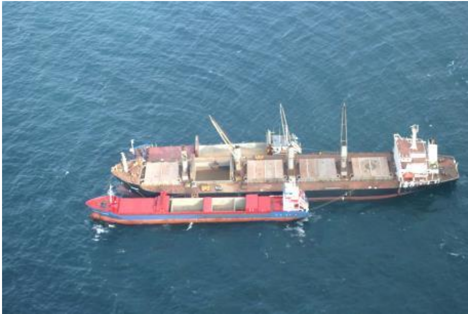
Figure 15. VICTORIA lightering the cargo Image: The Swedish Coast Guard.
