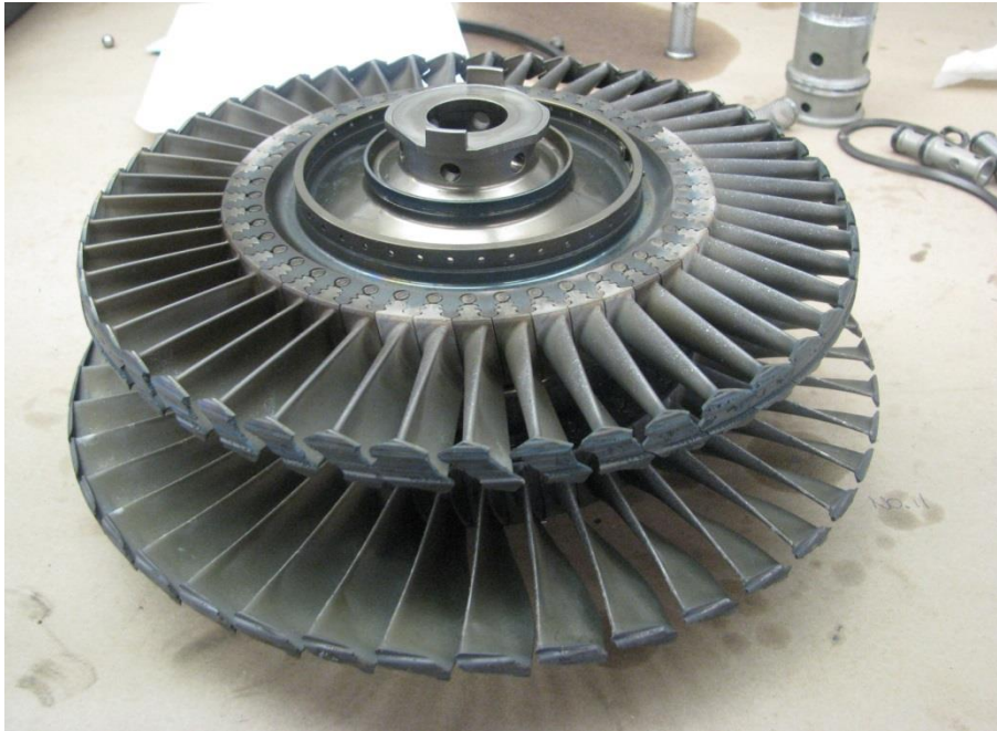
Figure 30. Damages to the turbine blades.
