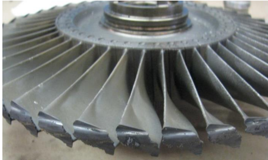
Figure 26. Second turbine section with damaged blade edges.
