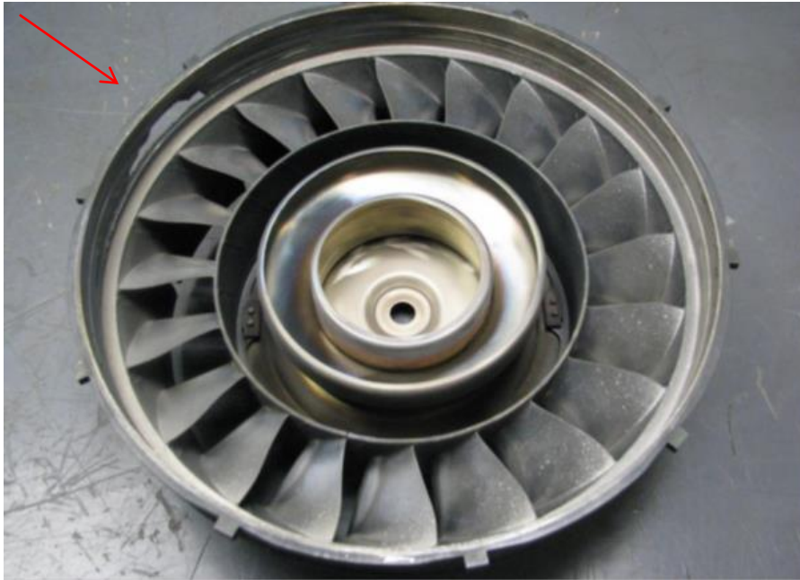
Figure 20. The casing for the first turbine stage, perforated at 10 o'clock.
