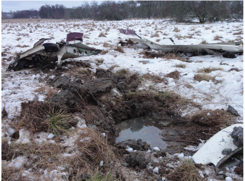
Figure 31. Picture from the scene of the accident showing leaked fuel.
