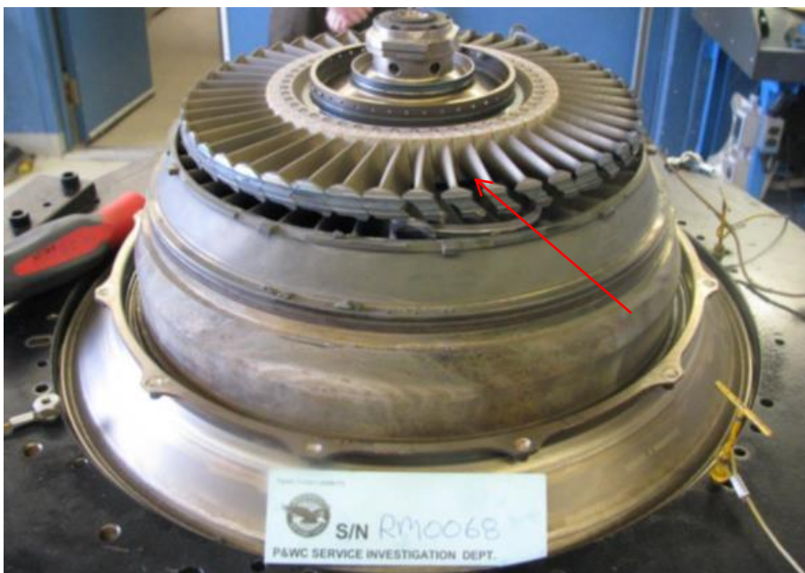
Figure 21. Damage to the blade tip shrouds in the first turbine stage.
