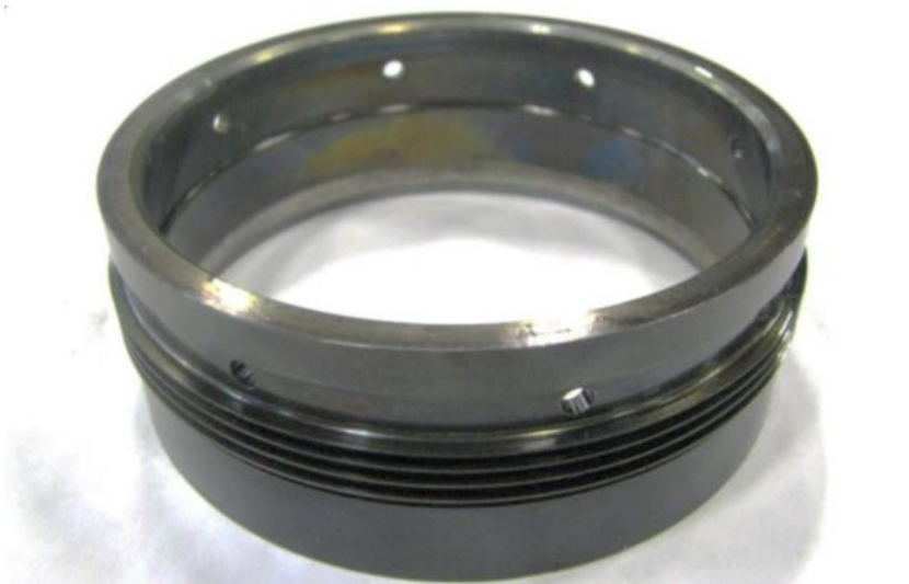
Figure 25. Comparison: New rotor section of a labyrinth seal.
