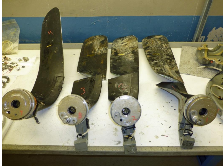
Figure 19. Examination of propeller blades.
