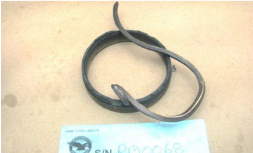
Figure 24. The broken rotor section of the labyrinth seal.
