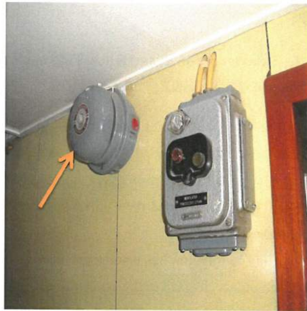
Photograph 31: The alarm-bell on the wall of the alleyway near the crew cabins; a photograph from a sister tug boat "Cyklop"
