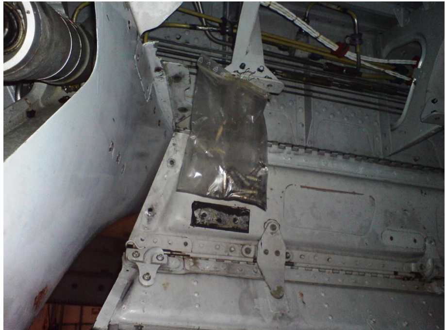
Photo 20: RH Bute door screws in bag, OY-KGZ.
