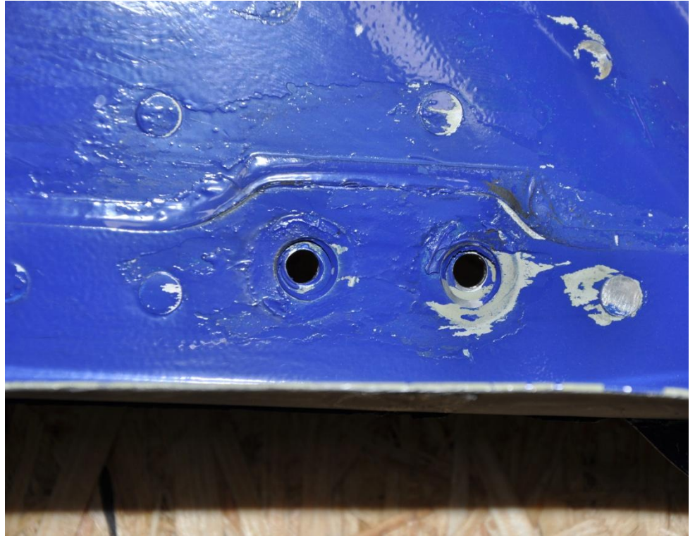
Photo 3: 2-NAS1203-4 position, RH fairing.
