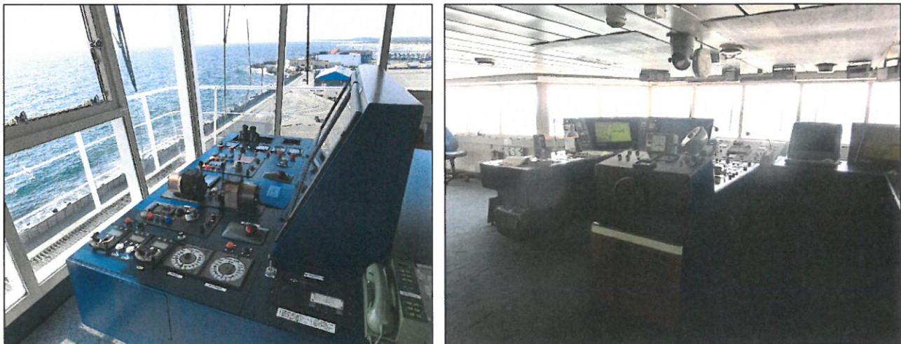
Figure 4: Port and centre steering consoles. Source: DMAIB
