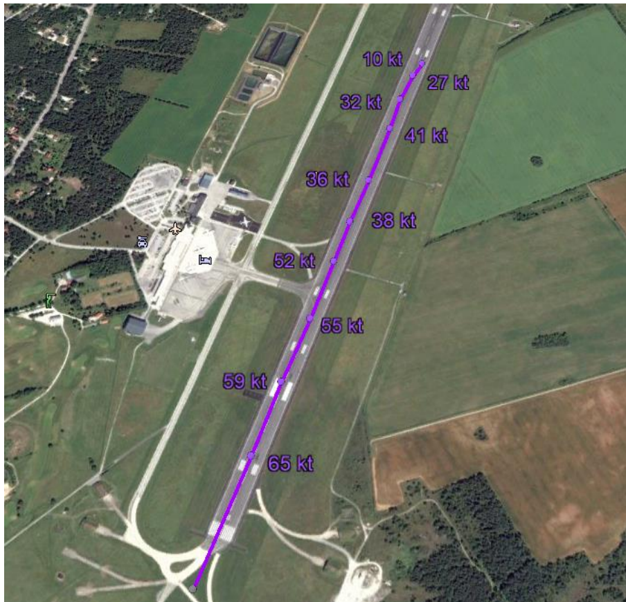
Figure 9. The Landing. Each point represents the average speed (ground speed) calculated from the previous point. Route and text inserted by SHK. Picture: Google Earth.
