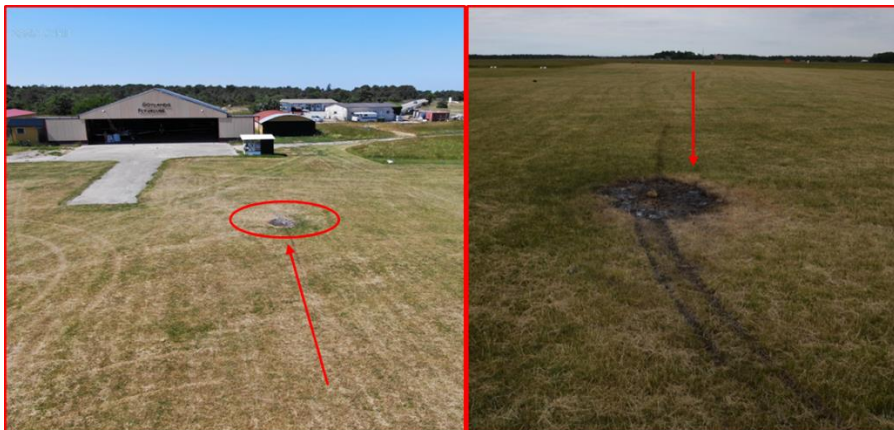
Figure 11. Left picture: Overview of the grass surface where the aircraft stopped. The arrow shows the direction of travel the last part before stopping. Red ring marks final position and marks in the grass after the fire. Right picture: Fire place and dark track in the grass after taxiing in and the arrow shows the direction of travel. Traces from the fire place on this side has been created after the fire was extinguished and the aircraft was moved.
