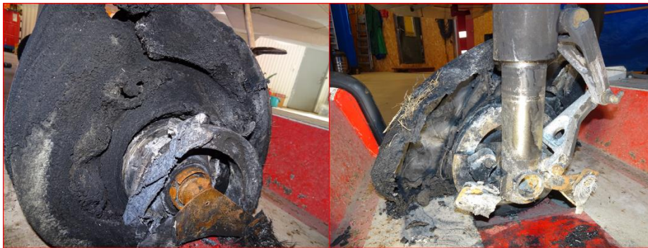
Figure 14. Pictures on the left landing gear, rim, tire and brake that had been ravaged by fire.
