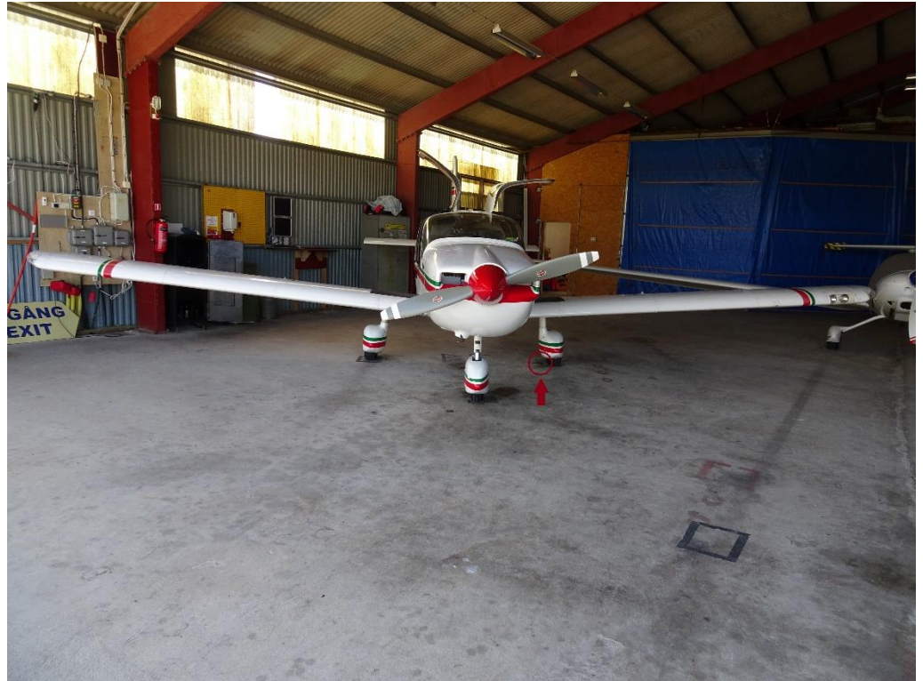
Figure 15. The parking in the hangar illustrated with another aircraft of the same model. At the left landing gear, the stain is marked with a red circle.
