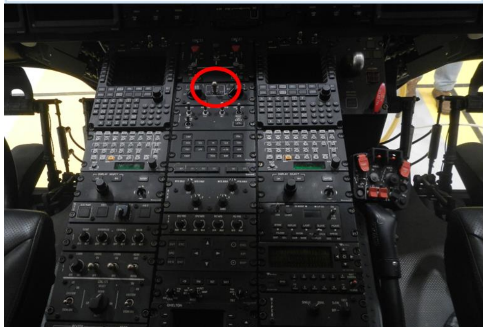
Figure 7. The red circle shows the design of the training mode switch. The panel is located on the centre console between the pilots.
