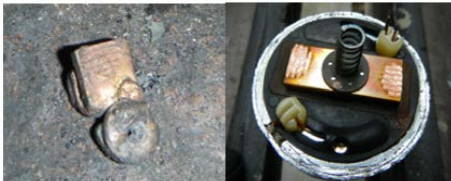
Figure 23. The short-circuited copper plate removed from the solenoid on the left and a copper plate from an undamaged starting motor of the same type on the right.
