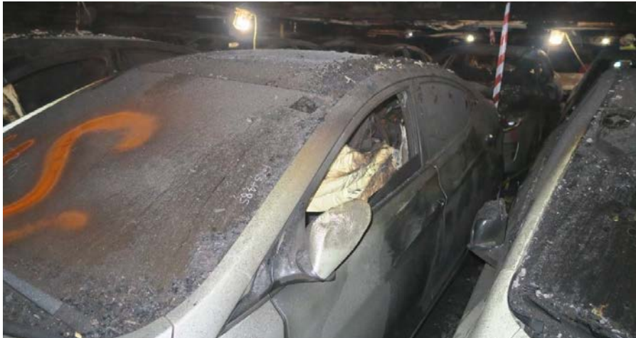
Figure 27. Rolled-down driver's window. Note the deployed airbag and the short distance between the cars.
