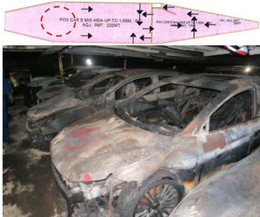
Figure 17. The likely starting point of the fire is in the area circled with a broken line on the deck drawing. Also shown in the image is the marking, the numbers on the hood, that was done on the cars in order to identify the different cars more easily.
