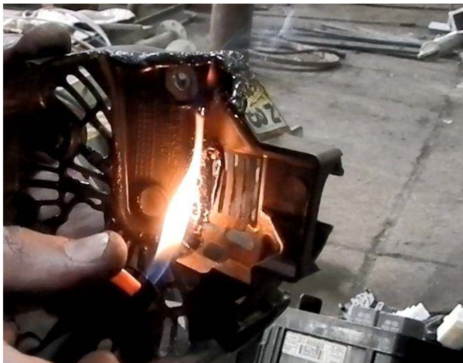
Figure 24. Example of one of the simple fire tests performed. The image shows the generator cover being tested. The cover could be ignited, but self-extinguished when the flame was removed.
