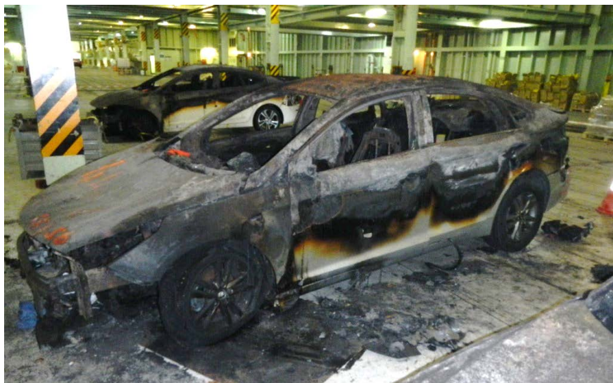
Figure 18. The fire pattern on the car where the fire likely started. In this image, the cars have been moved from deck 1 to an undamaged deck higher up in the vessel for further investigation.
