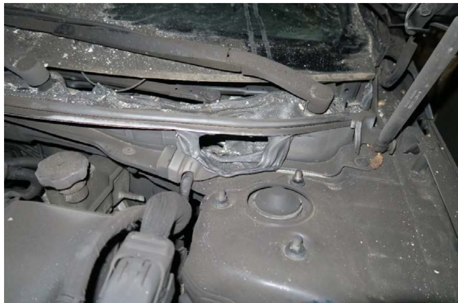
Figure 26. Openings between the engine and passenger compartments, where the plastic has melted.
