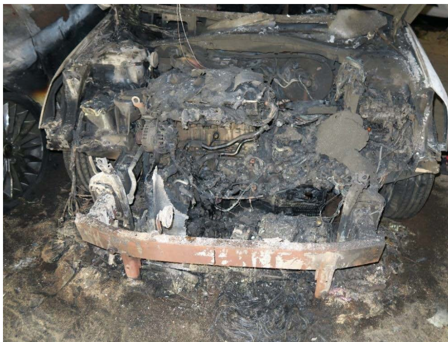
Figure 19. The engine room of the car where the fire likely started.
