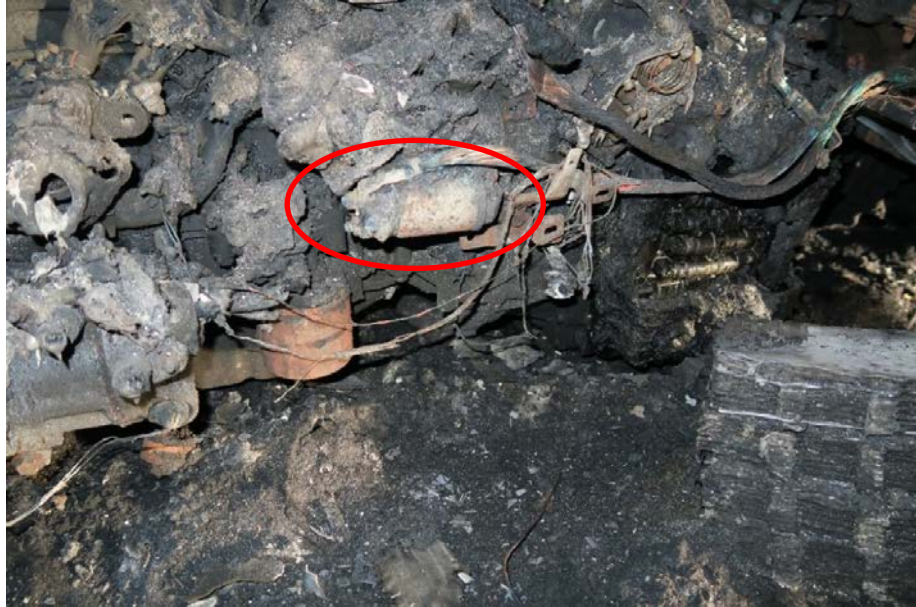
Figure 20. The solenoid of the starting motor where the fire most likely started.
