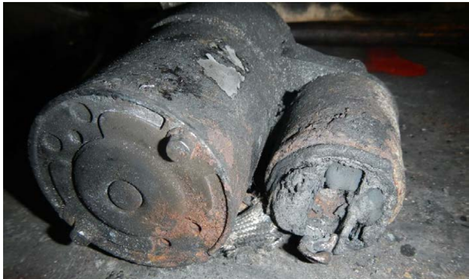
Figure 21. The starting motor with the solenoid to the right.
