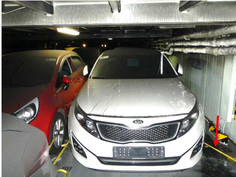
Figure 12. The cars were parked very close together. Also visible in the photo are the yellow lashings between the deck and the wheels, see arrow on the right.
