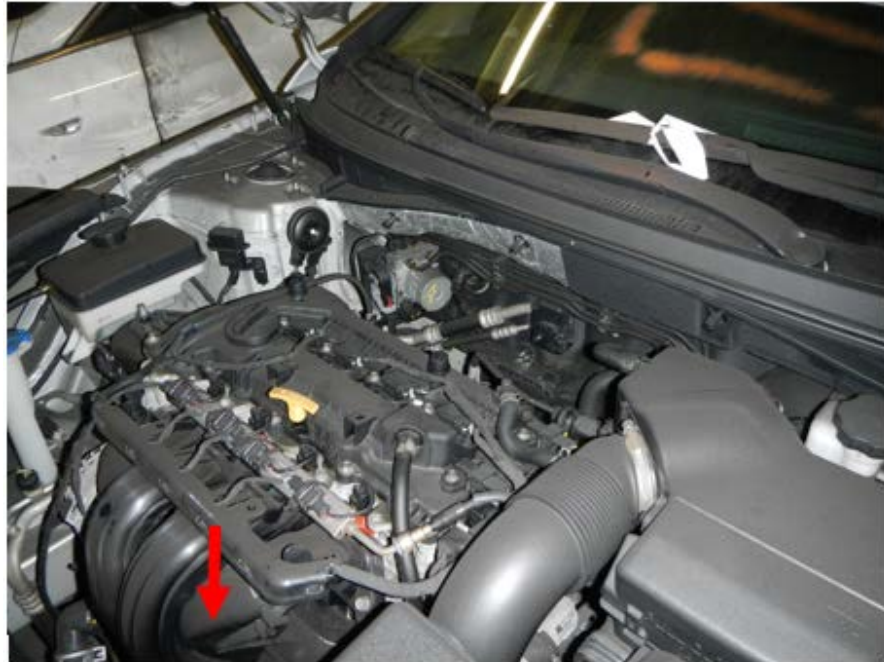
Figure 25. The engine compartment of the reference car. The arrow marks the plastic inlet pipe and the approximate positions of the solenoid and the starting motor below it.
