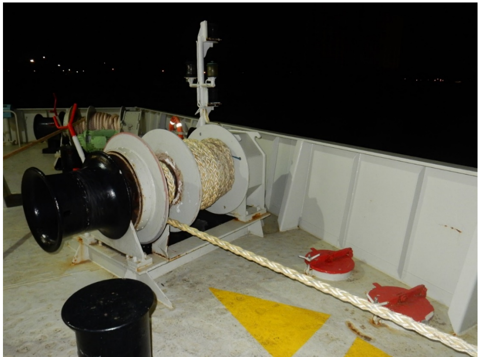
Figure 12. Mooring winch with the fixed regular mooring line.
