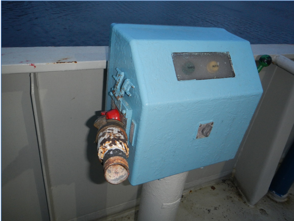
Figure 18. The lever locked on high speed with the water adapter.
