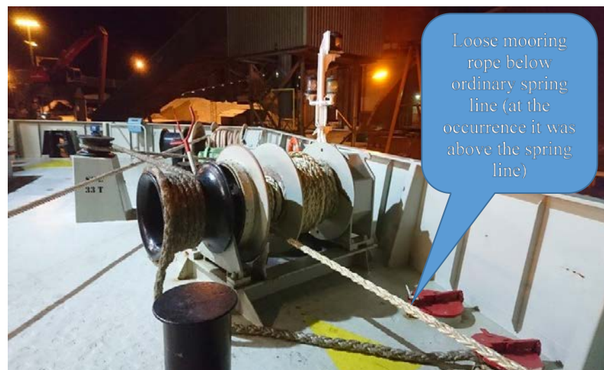
Figure 9. Mooring winch and hatches to rope store.
