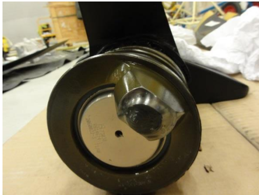
Figure 1 and 2. The failed trunnion pin.
