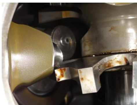
Figure 3 and 4. The bent actuator plate.
