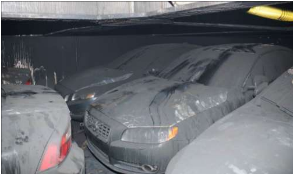
Figure 9: Cars severely fouled by soot
