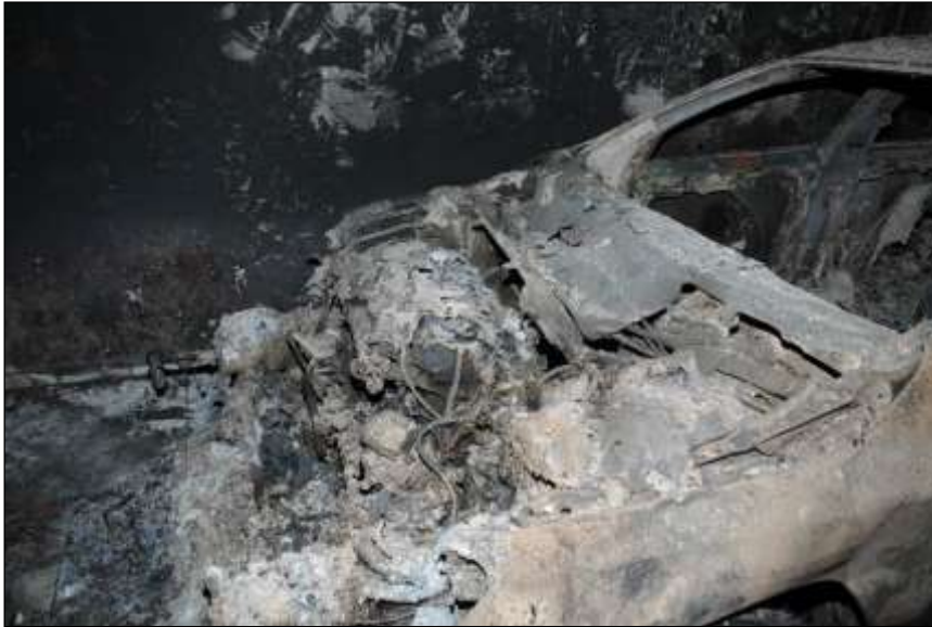
Figure 55: Engine compartment of a car destroyed by metal fire
