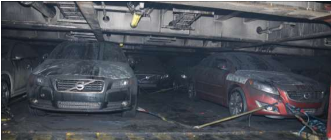
Figure 53: Vehicles in the outer area fouled by soot
