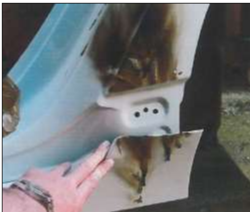
Figure 90: Ignition of the door sill (1) 62
