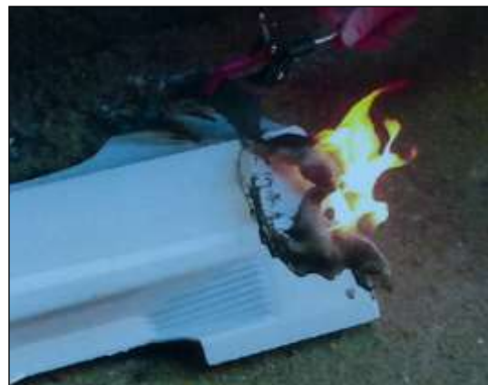
Figure 91: Ignition of the door sill (2) 63
