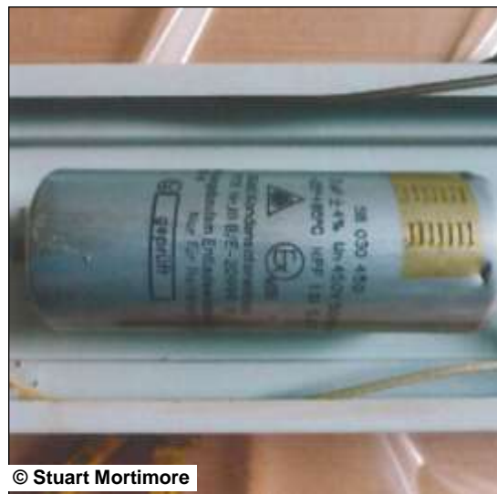
Figure 87: Lamp socket and capacitor 59
