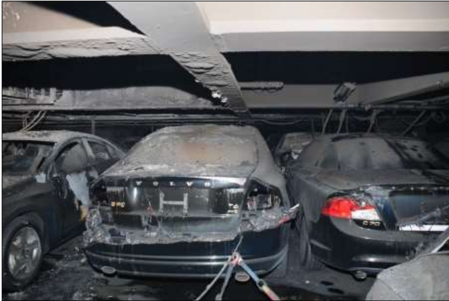
Figure 51: Destroyed plastic parts (in this case the rear lights) on the vehicles
