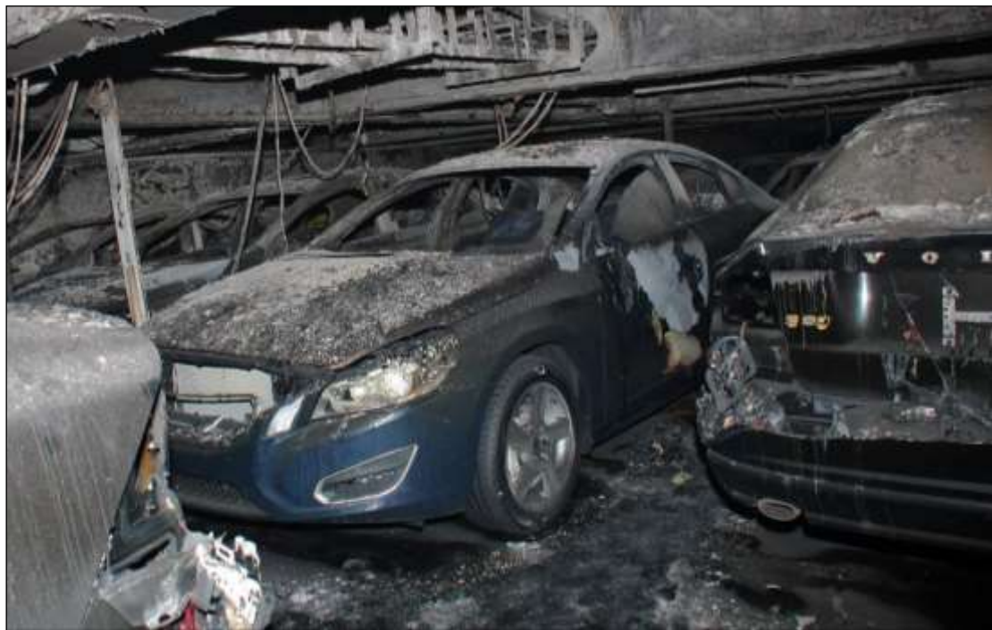
Figure 8: Cars damaged to varying degrees by the heat
