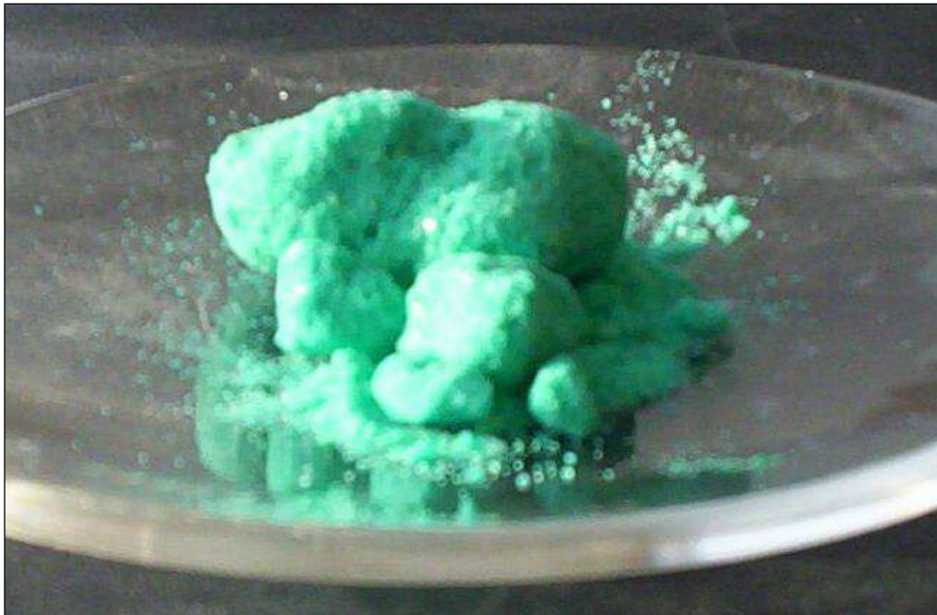
Figure 112: Copper(II) chloride dihydrate \text{CuCl}_2 \cdot 2 \text{H}_2\text{O}
