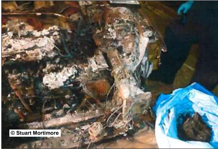
Figure 99: Burnt out engine compartment (example) 72
