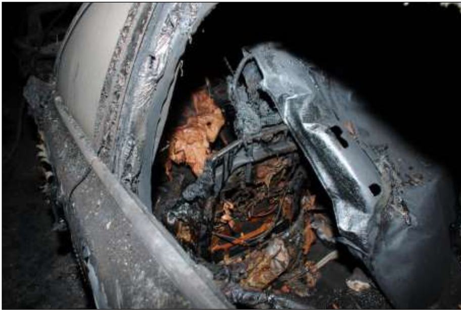
Figure 60: Fragments of a triggered air bag inside a car
