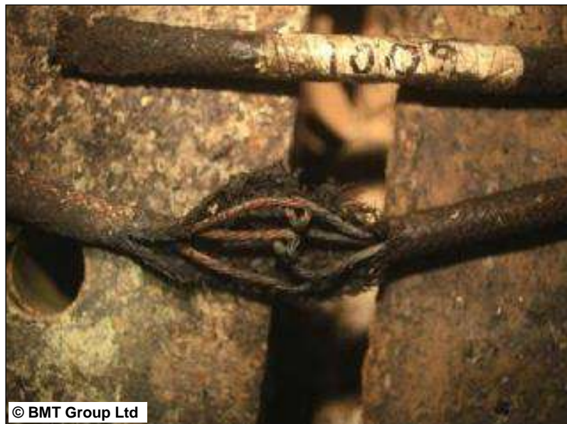
Figure 70: Example of metal conductor within the insulation 43
