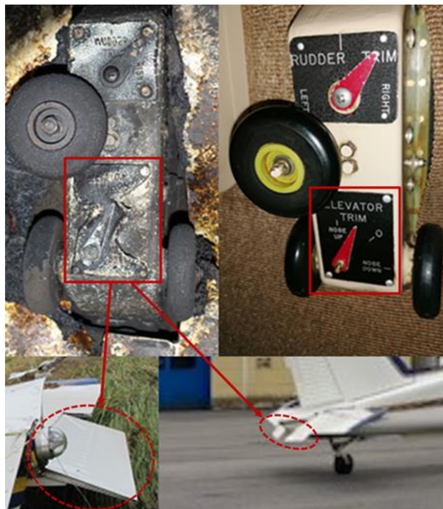
Figure 30. The pictures present the elevator trim indication and trim tab position before and after the accident. Lower right image: Private person.
