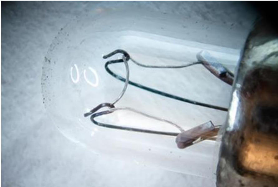
Figure 43. Intact filament without deformation.
