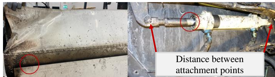
Figure 34. The left picture shows soot trails around the wing and wing flap. The right picture shows the operating cylinder and attachment points. Soot edge circled in red.
