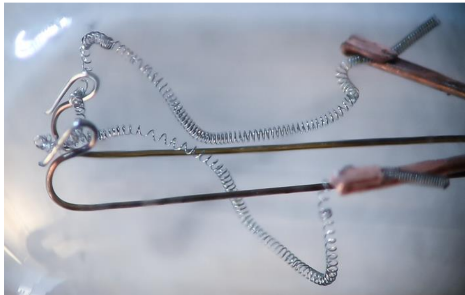
Figure 42. Enlargement of an image of the stall warning light bulb. The picture shows the deformed filament.
