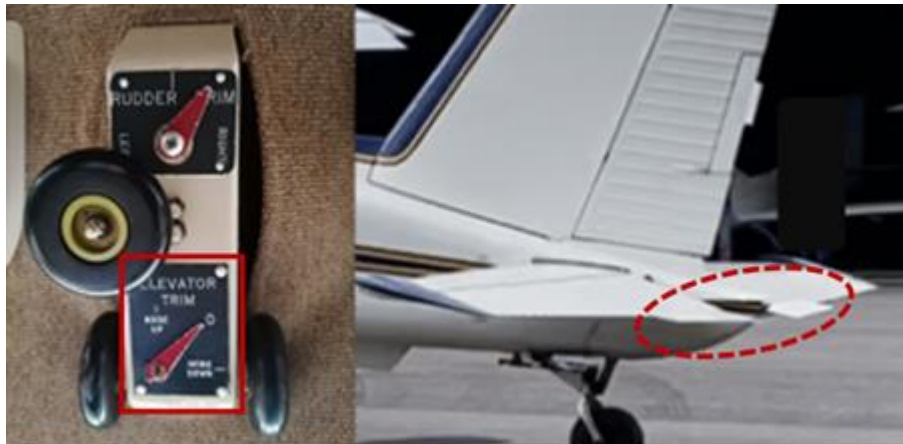
Figure 31 Trim panel setting and elevator trim tab position before take-off with a pilot and parachutists on board. Right picture: Örebro Skydivers Club.
