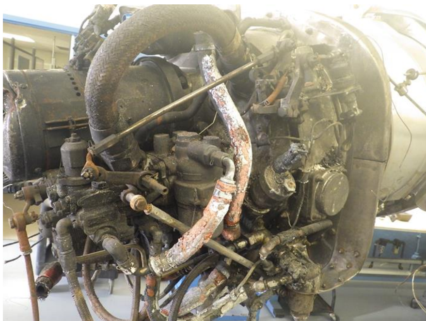
Figure 36. The auxiliary gearbox had been exposed to fire. Photo: Pratt & Whitney Canada Corp.
