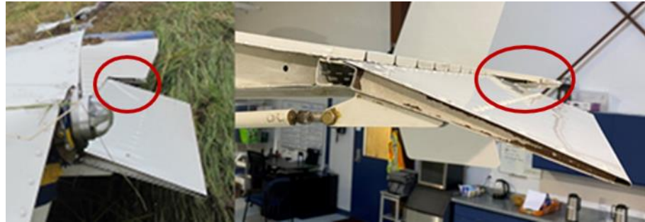
Figure 33. The left part of the picture shows the position of the elevator trim tab after the accident. The right part shows the elevator trim tab position at 16.5 degrees nose up according to the type certificate holder.
