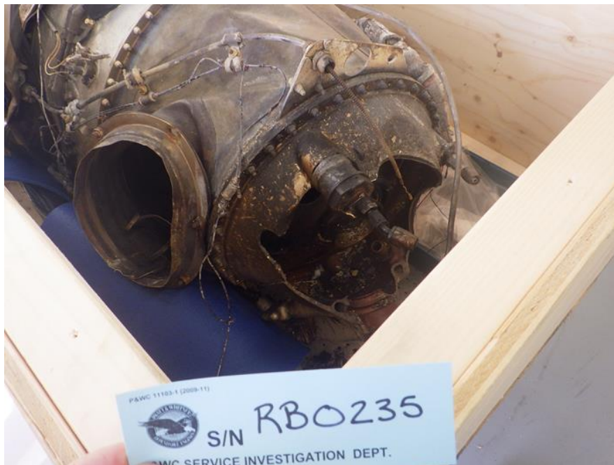
Figure 35. The front gearbox housing was cracked, exposing the internal components. Photo: Pratt & Whitney Canada Corp.
