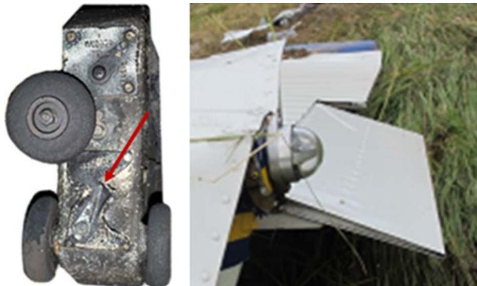
Figure 25. The left picture shows the trim panel where the arrow points to the set position of the elevator trim. The right picture shows the corresponding position on the right elevator trim tab.
