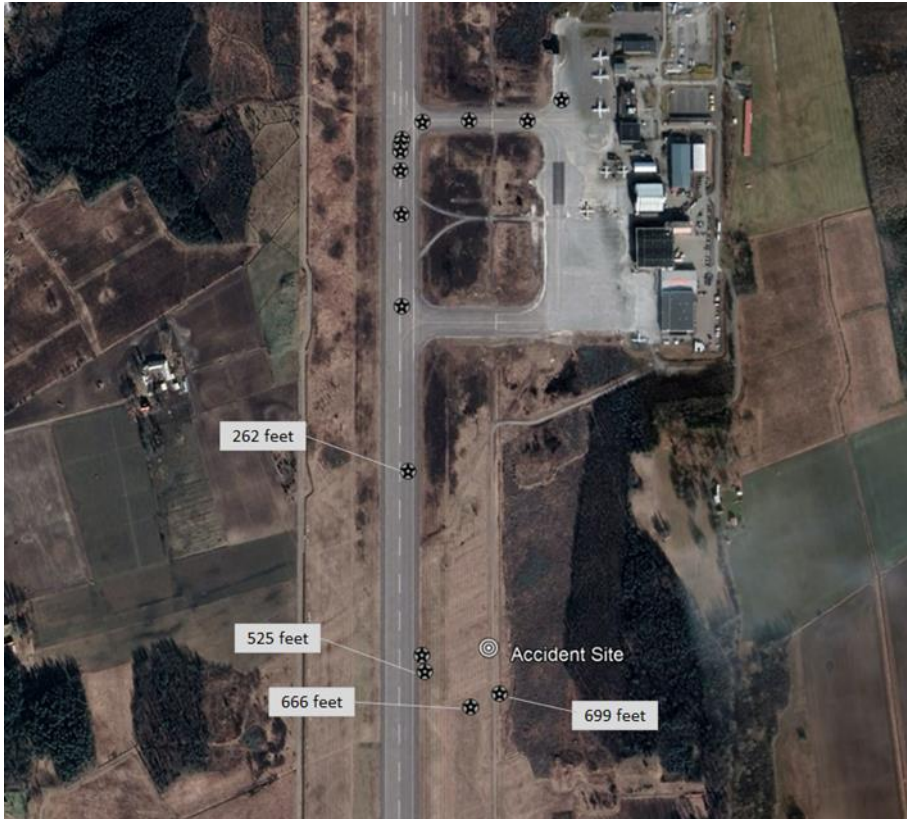
Figure 9. Aircraft position and altitude recordings from GPS. Image: Google Earth with markings inserted by SHK.
