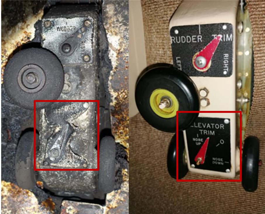
Figure 17. The picture on the left shows the trim panel from the wreckage and the picture on the right shows an intact panel with the same setting. The red boxes show the elevator trim.
