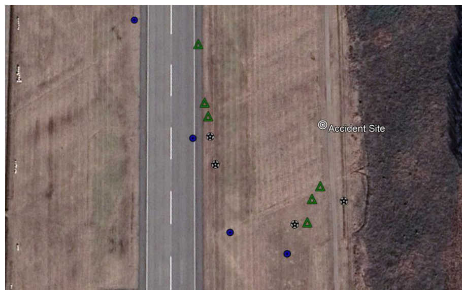
Figure 14. Blue markings show radar data, green markings show ADS-B data and grey markings with a star show GPS data. Image: Google Earth with markings inserted by SHK.
