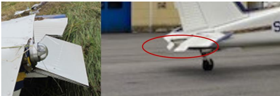
Figure 18. The left image shows the position of the elevator trim after the accident and the right image is taken from a surveillance camera when the aircraft is taxiing out to the runway.
