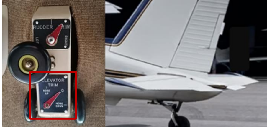
Figure 19. The left part of the picture shows a trim setting which, according to other pilots, is normal for take-off with a pilot and eight parachutists on board. The red box shows the elevator trim. The right part shows the position of the rudder before one of the previous flights during the day.
