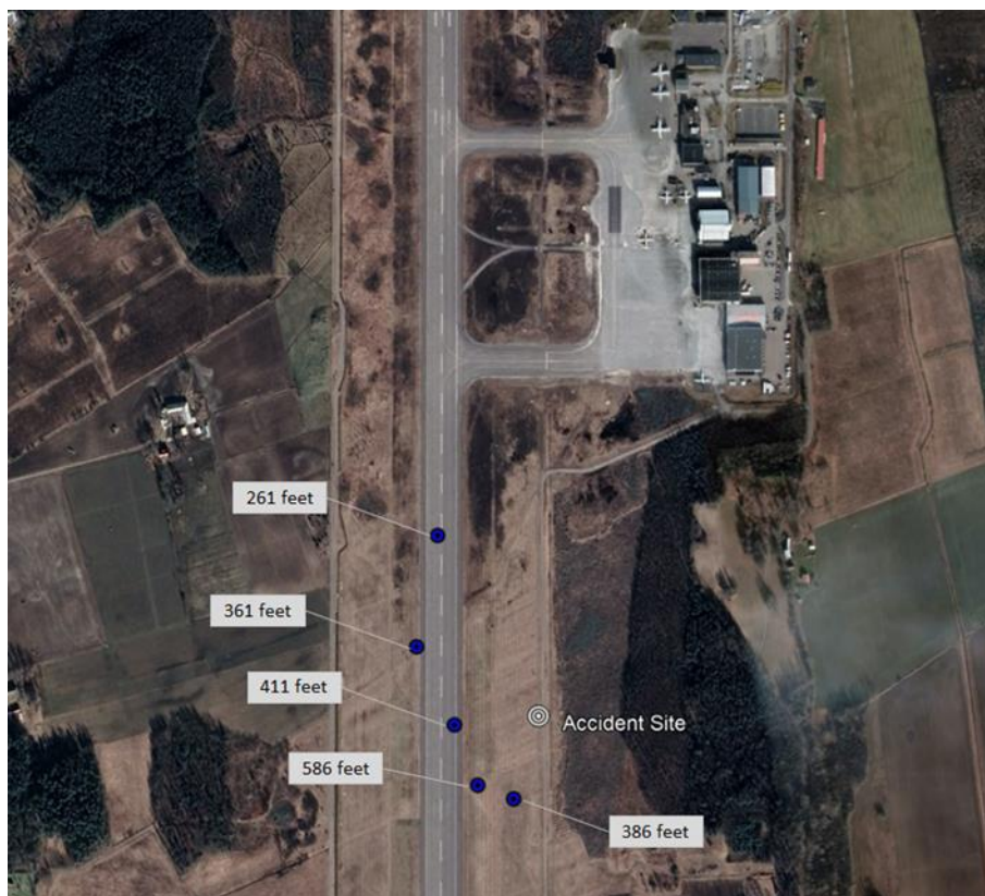
Figure 6. The aircraft's position registrations from Askersund's radar. Specified altitudes are adjusted for atmospheric pressure reduced to mean sea level (QNH) Image: Google Earth with markings inserted by SHK.
