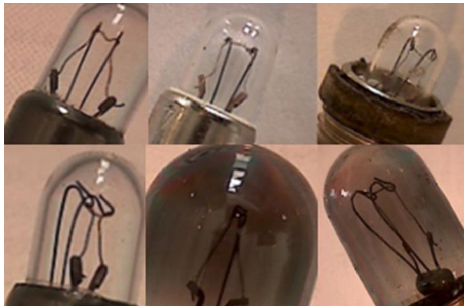
Figure 21. The filaments of these light bulbs were intact, indicating that they were not illuminated. From the top left row: Beta fail, Pitch position and Chip detect. Bottom row: Generator warning, Left low fuel pressure and Right low fuel pressure.
