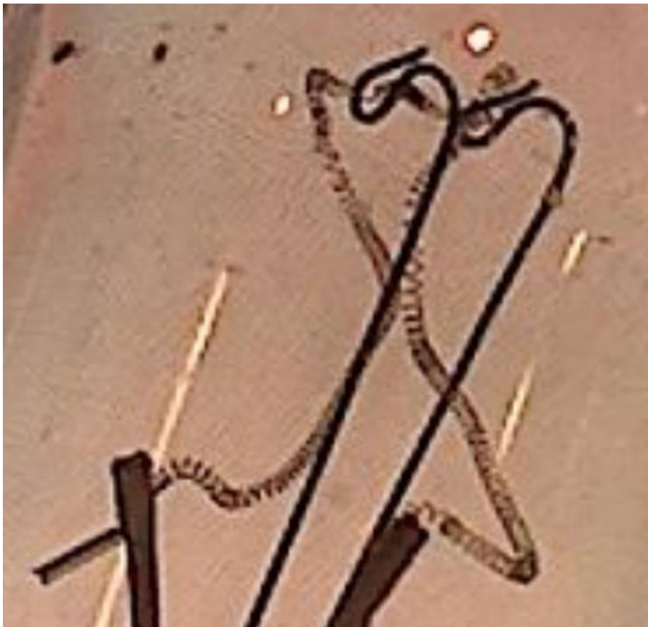
Figure 20. Enlargement of an image on the stall warning light bulb. The picture shows the deformed filament.
