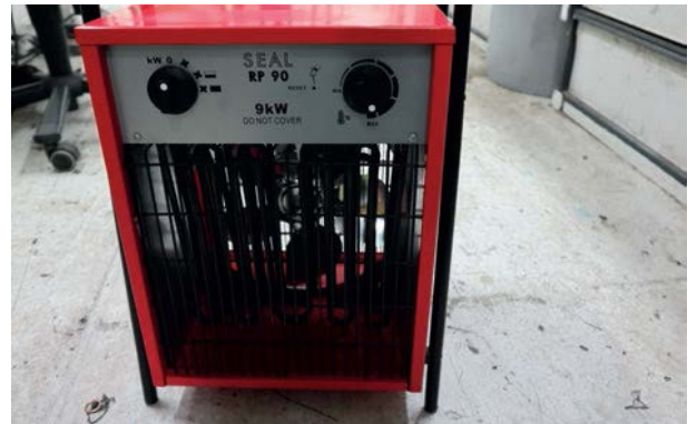
9 Kw electric heater. (Source: Dutch Safety Board)
