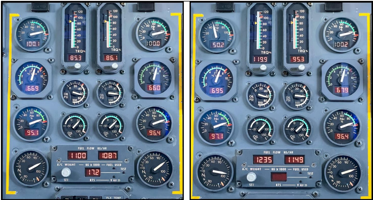
Figure 3. On the left, engine indications during a normal takeoff. On the right, the left propeller is feathered, but the engine is operating. (Figures: Gabriel Leigh / Fliht radar24, edited by SIAF).
