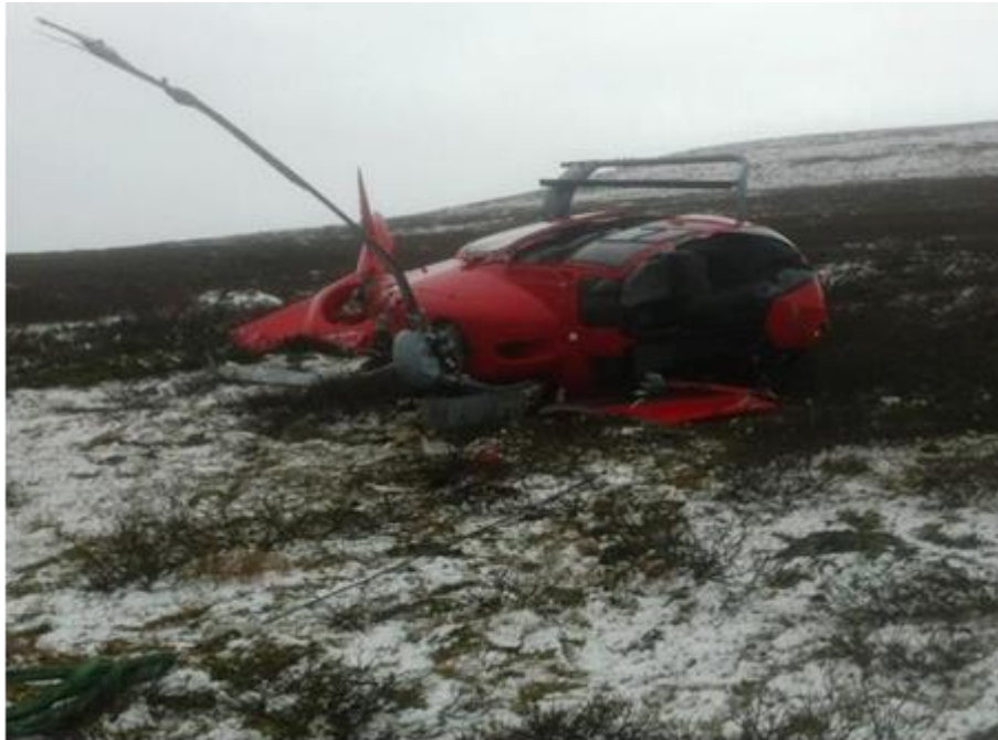
Figure 4. The helicopter at the crash site with sling load cable and straps in the foreground (Photo Kallax Flyg AB).
