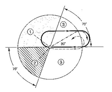
When two ADFs are installed onboard the aircraft, one of these can be selected to the inner locator after outer locator passage, in this case F. By doing so the possibility is increased of obtaining an indication concerning the position of the aircraft laterally with respect to the final approach course, as now one of the needles is pointing forward and the other to the rear.
