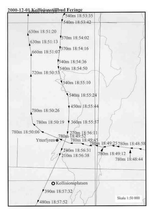
Note. Between the time points 18:56:38 and 18:57:32 the aircraft has been at such a low altitude that radar echoes have not been noted.
