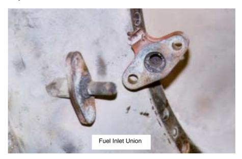
The coke was analysed by CSM using spectral analysis and it was determined that it contained calcium, carbon, barium, magnesium, fluorine, in addition to traces of iron, sulphur and oxygen. According to their assessment these basic elements are not derived solely from the burning of jet fuel. Their most probable source would be from the carbonised remains of spent rubber and/or plastic.
