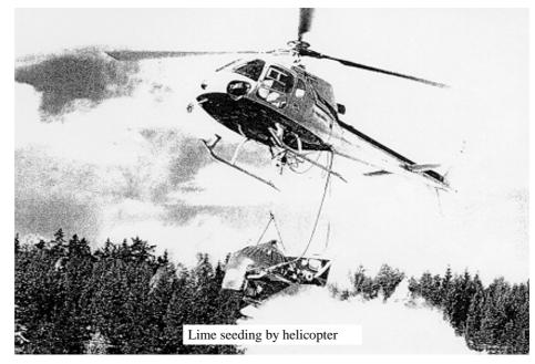
The specially designed lime spreader used in seeding operations has a cylindrical form and is made of fibre glass strengthened plastic. It is slung beneath the helicopter using two cables that are connected to the cargo hook under the fuselage. The pilot is able to open and close the lime release valve on the spreader from the cockpit
