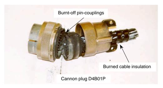
The investigation also showed that several of the contact pins were discolored due to the overheating and that the insulating material between the pins in the cannon plug had been affected by high temperature and had also been discolored. This all points to the fact that the source of heat generation was not external in connection with the fire but took place within the electrical pin couplings during an extended period of time.
