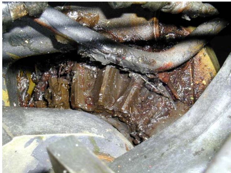
Rack segment and damaged hydraulic line
