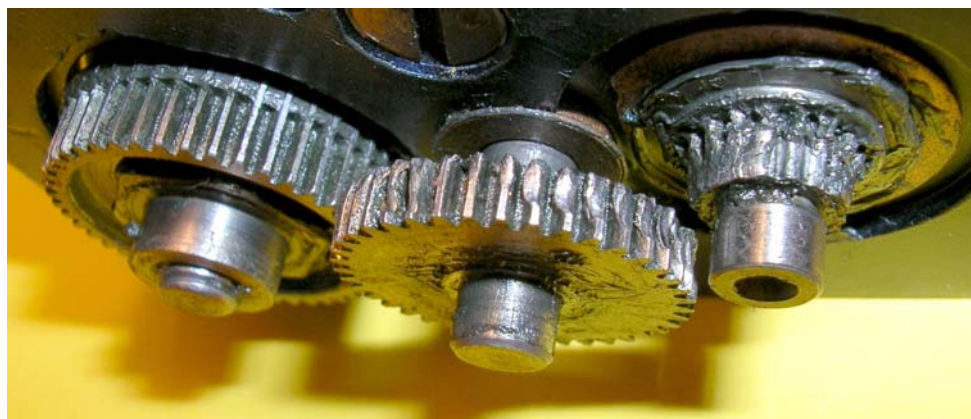
Gearwheels in the trim actuator gearbox
