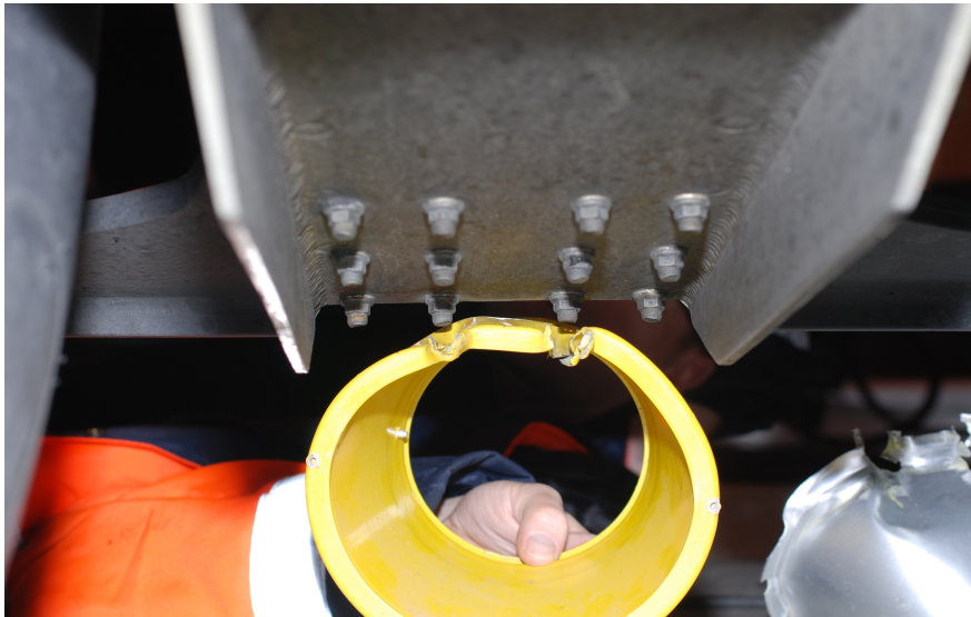
Fig.7. Detail view of part of the MD-83 landing gear and lamp housing C1:4.
