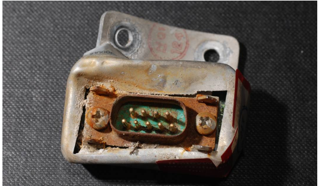
Fig 12. The autopilot's KCM 100 unit. Photograph source: SHK.
