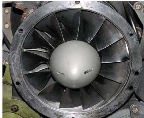
First compressor stage
