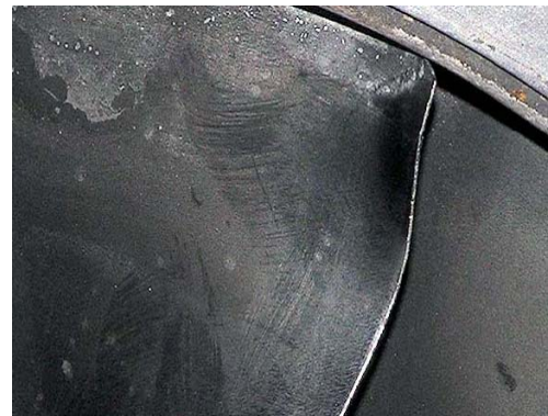
Damage to the compressor blade
