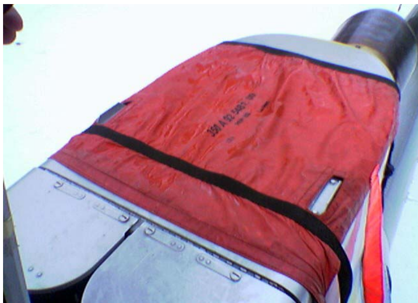
Tarpaulin covering the engine air intake
