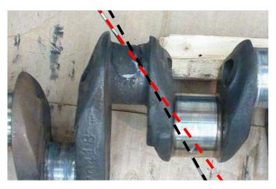
Directions of two drill holes in the crankshaft
