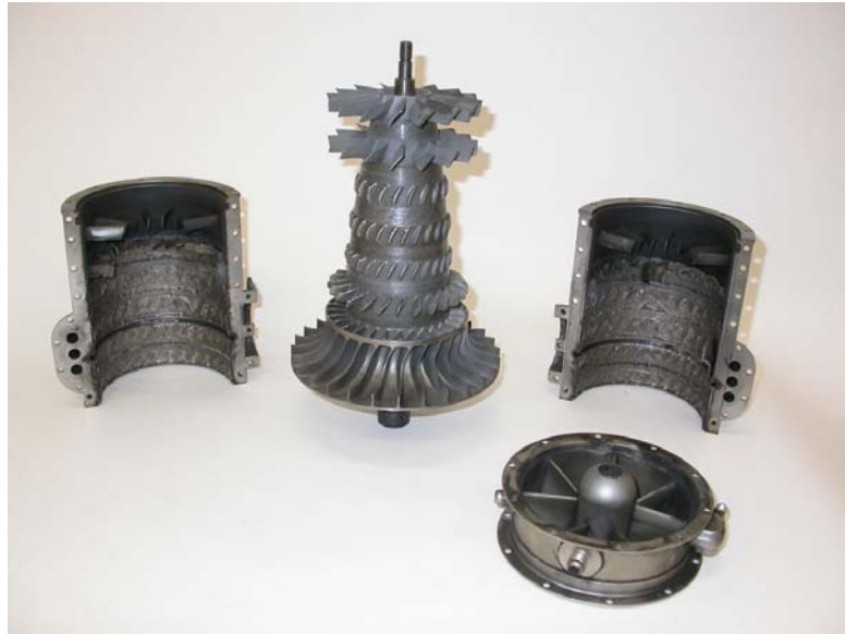
Figure 2. Principal parts of the compressor after dismantling.
