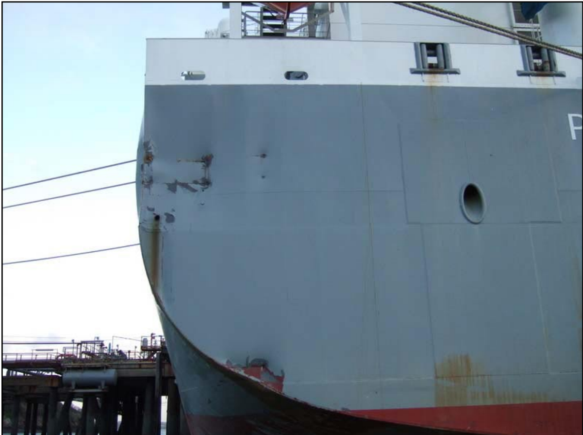
Damage to stern of Prospero by jetty dolphins, from aft.
