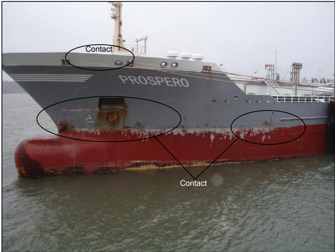
Bow of Prospero , showing damage by jetty and gantry
